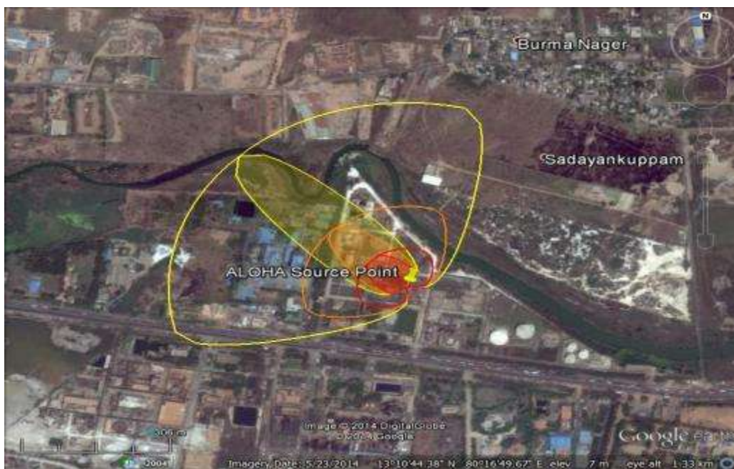
Figure 2 Google Image of Threat Zone- Toxic area Vapor cloud for Propylene Oxide
