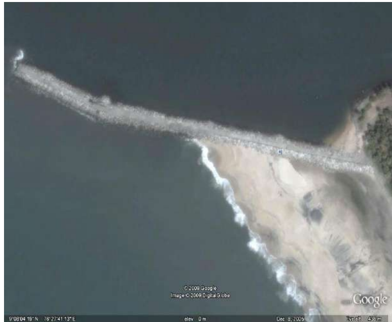
Fig 5.5 Beach formation due to construction of groyne.
