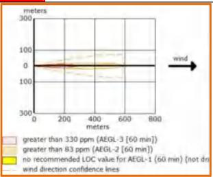
THREAT ZONE: Model Run: Gaussian **Red** : 284 meters --- (330 ppm = AEGL-3 [60 min]) Orange: 594 meters --- (83 ppm = AEGL-2 [60 min])
