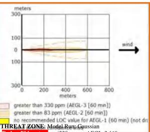
Red : 284 meters --- (330 ppm = AEGL-3 [60 min]) Orange: 594 meters --- (83 ppm = AEGL-2 [60 min])
