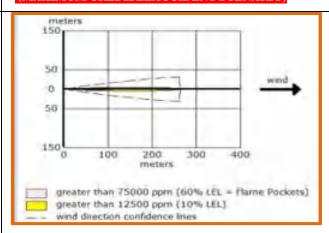
THREAT ZONE: Threat Modeled: Flammable Area of Vapor Cloud Model Run: Gaussian
