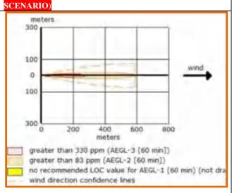
THREAT ZONE: Model Run: Gaussian Red : 284 meters --- (330 ppm = AEGL-3 [60 min])Orange: 594 meters --- (83 ppm = AEGL-2 [60 min]) Yellow: no recommended LOC value --- (N/A = AEGL-1 [60
