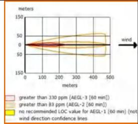
THREAT ZONE: Model Run: Gaussian Red: 230 meters --- (330 ppm = AEGL-3 [60 min]) Orange: 476 meters --- (83 ppm =
