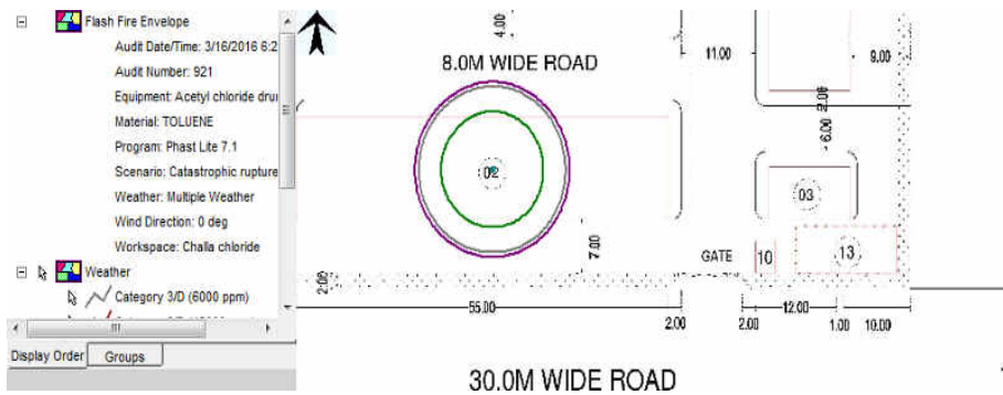
Fig.11.26 Flash Fire of Acetyl chloride by Catastrophic Rupture
