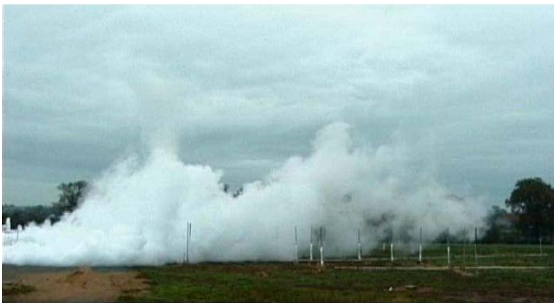
Figure 5.3: Dispersion of LNG vapours by wind on field
