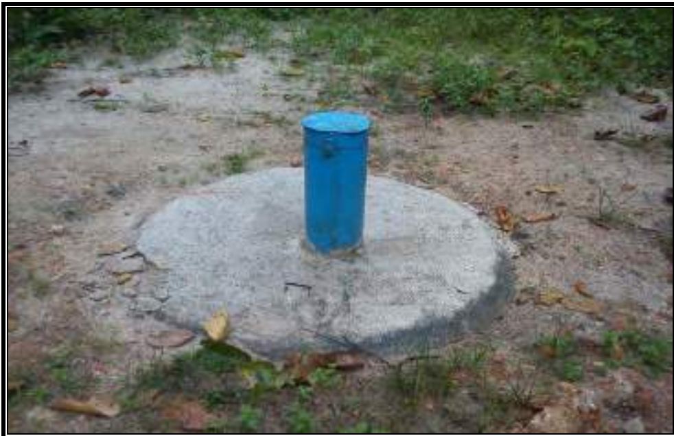
Photo 2: Piezometer constructed in and around Jagannath OCP, Talcher coalfield, Odisha.
