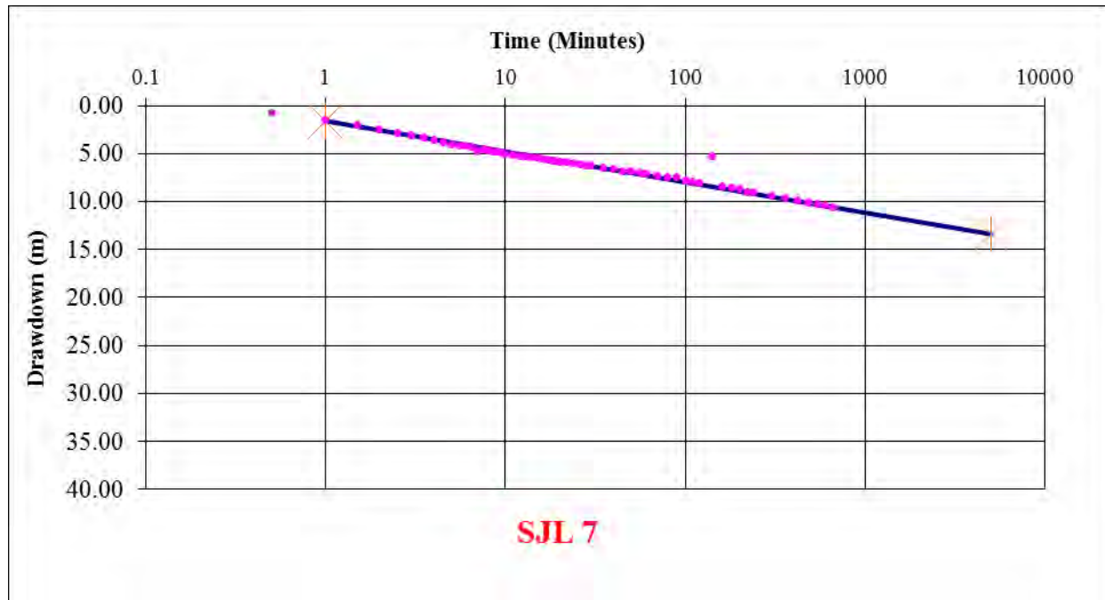
Plot 11: Time drawdown plot for piezometer no SJL 7 around Jagannath OCP, Talcher coalfield, Odisha.
