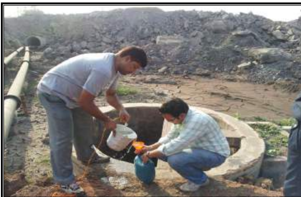
Photo 8: CMPDI team collecting groundwater sample from open dug well in and around Jagannath OCP, Talcher coalfield, Odisha.
