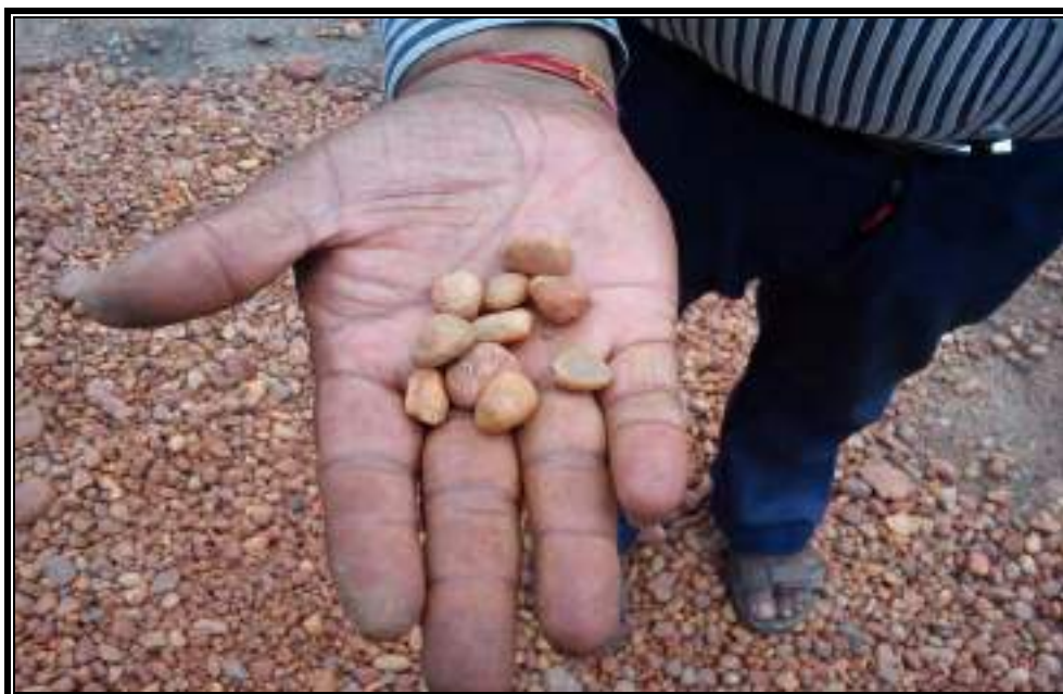
Photo 4: Gravels used for piezometer construction in and around Jagannath OCP, Talcher coalfield, Odisha.
