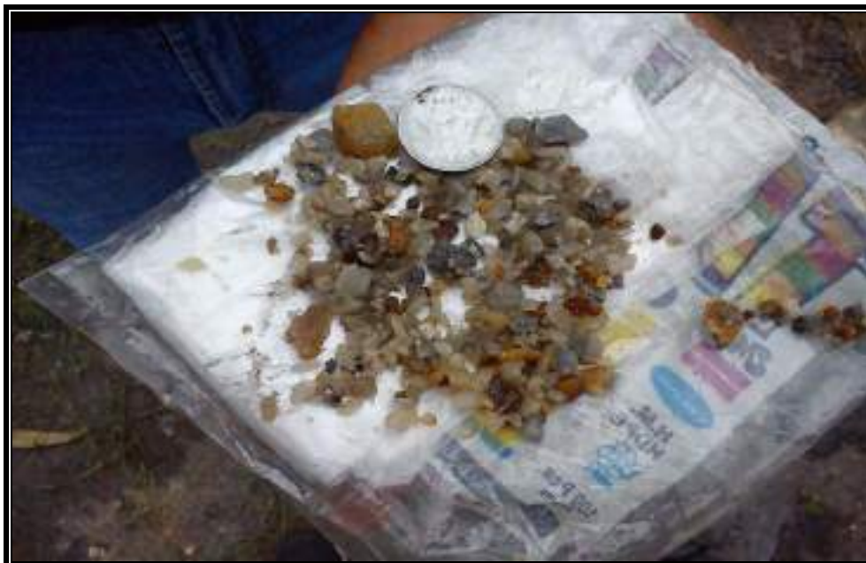
Photo 3: Drilling cutting sample at piezometer location in and around Jagannath OCP, Talcher coalfield, Odisha.
