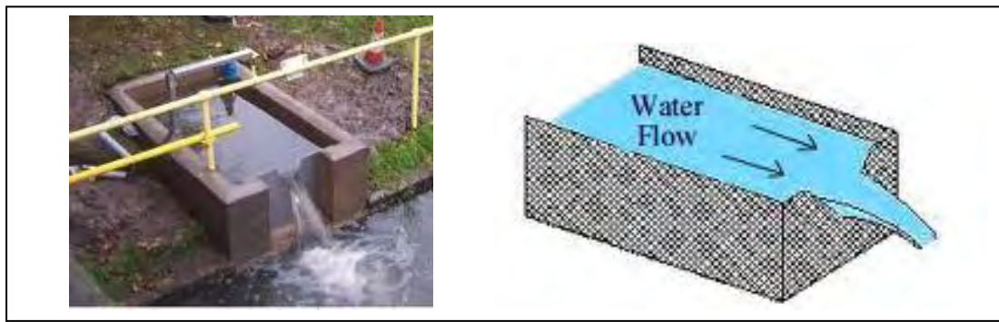
Figure-7: V-Notch arrangement for measuring Discharge
