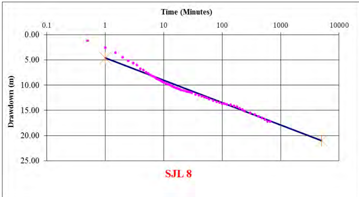
Plot 12: Time drawdown plot for piezometer no SJL 8 around Jagannath OCP, Talcher coalfield, Odisha.
