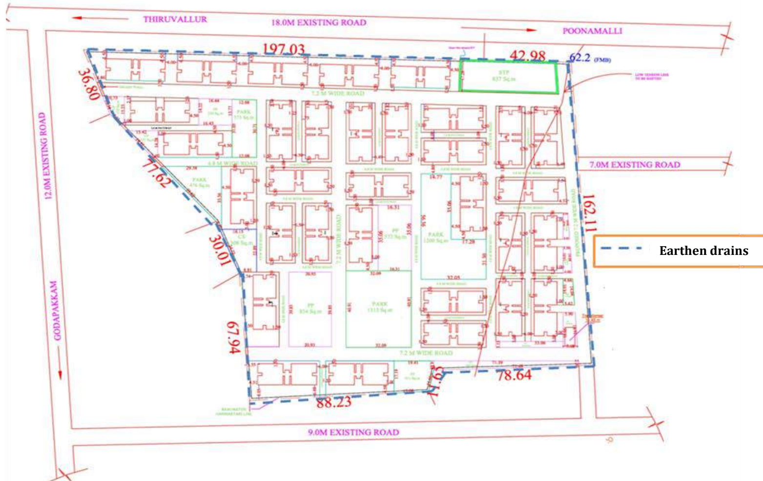
Figure 3.4 - Rain Water Harvesting Layout
