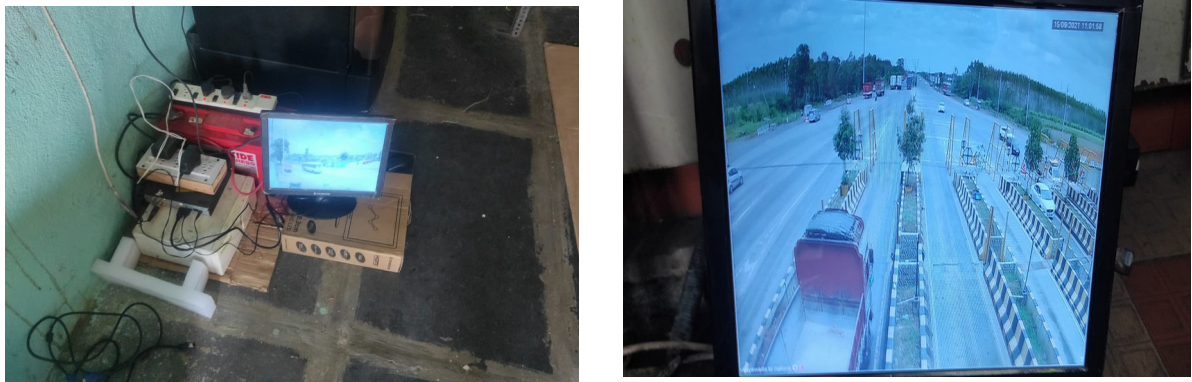
Figure-9.3: TVC survey using ATCC at various survey locations
