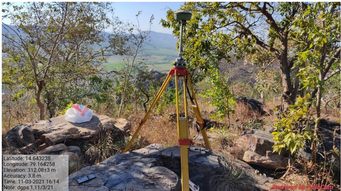
Photo 5-1: Establishment of GCP using DGPS
