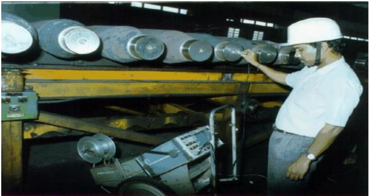
FIGURE 3.12: ULTRASONIC TESTING OF AXLE MAGNETIC PARTICLE TESTING
