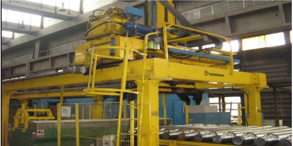
FIGURE 3.11: M/s. DANOBAT CNC MACHINES FOR MACHINING AXLES
