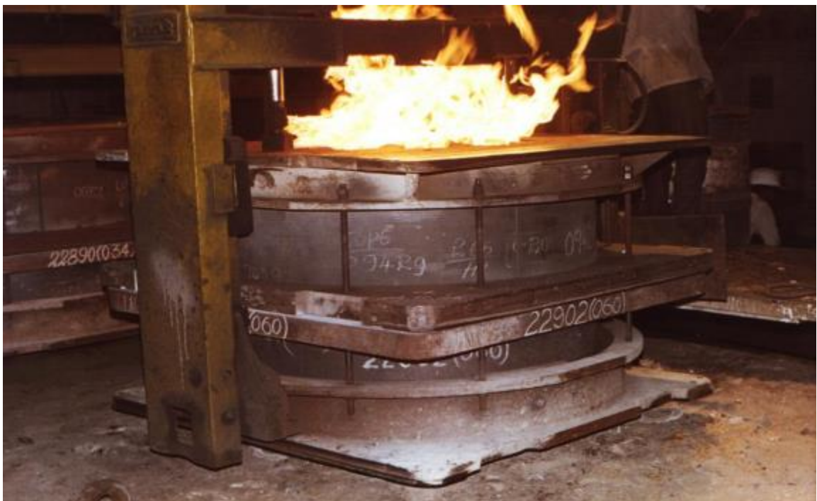
FIGURE 3.6: MOLTEN METAL POURING IN TO MOULD BOX
