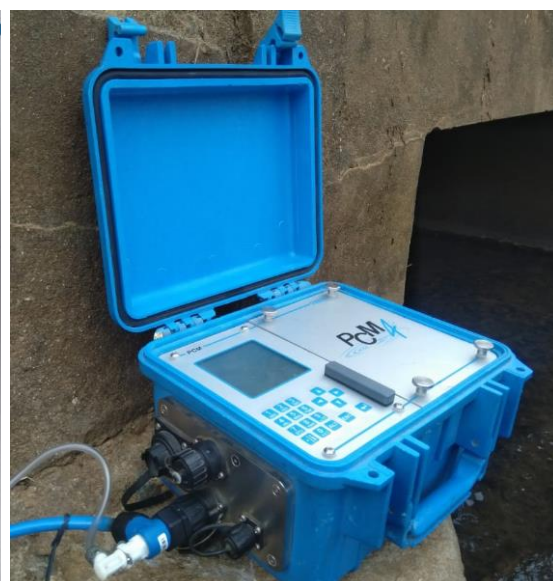
Installation & Calibration of Gauging Equipment (Nivuflow 750 transmitter with ultrasonic wedge sensor)
