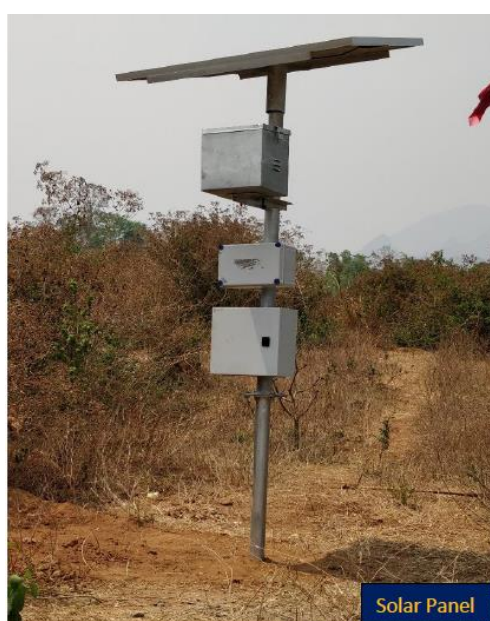
Solar Powered Equipment for Gauging Equipment
