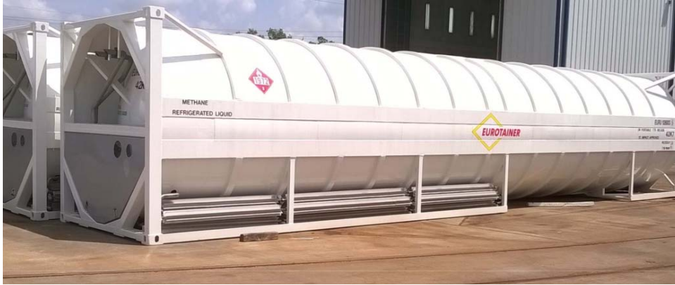
Figure: Example of Iso-container for storage of LNG
