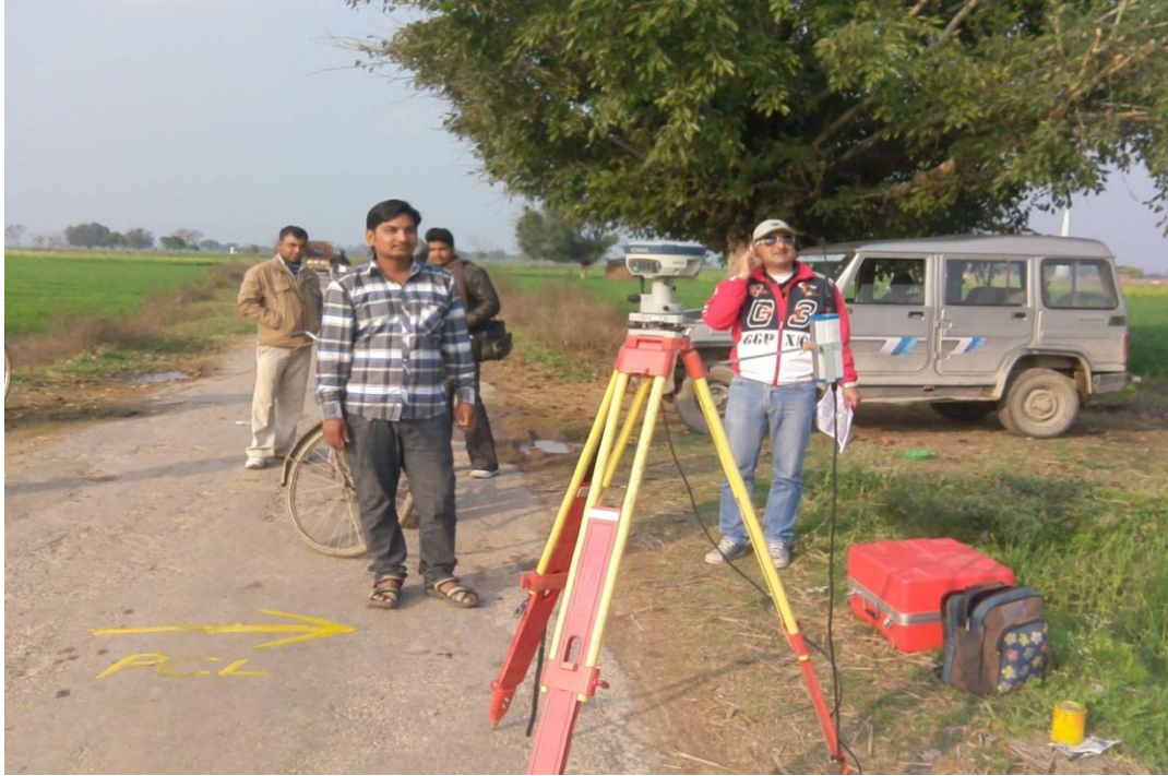
Survey in progress by DGPS
