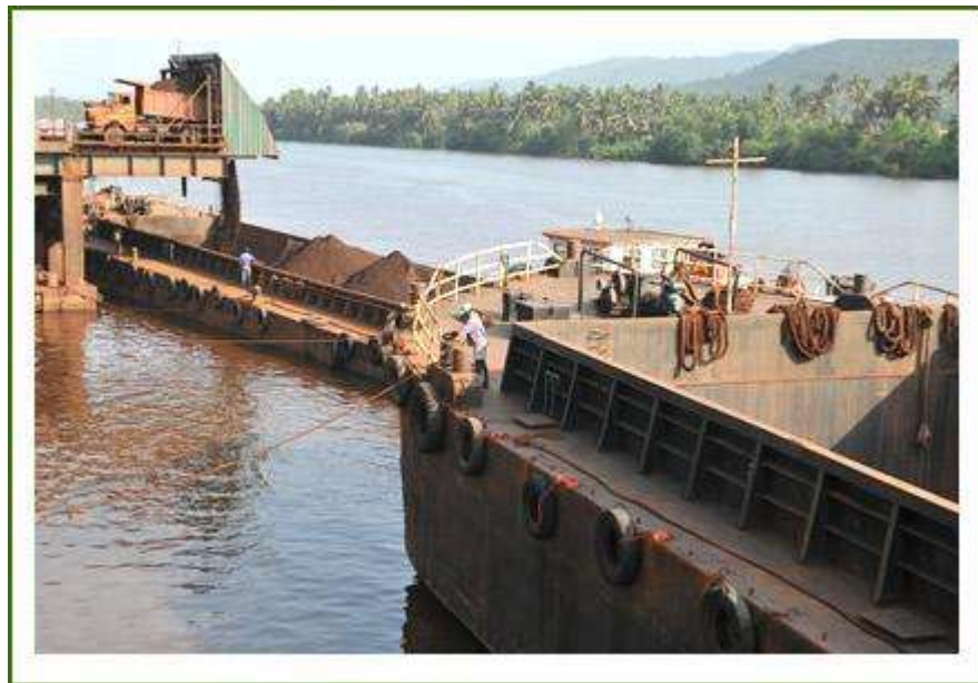
Fig.11: Iron ore loading from truck to barge at Jetty
