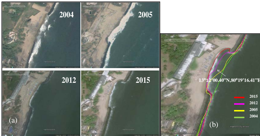
Fig 1. 32a and b. Shoreline behaviour near the termination of seawalls
