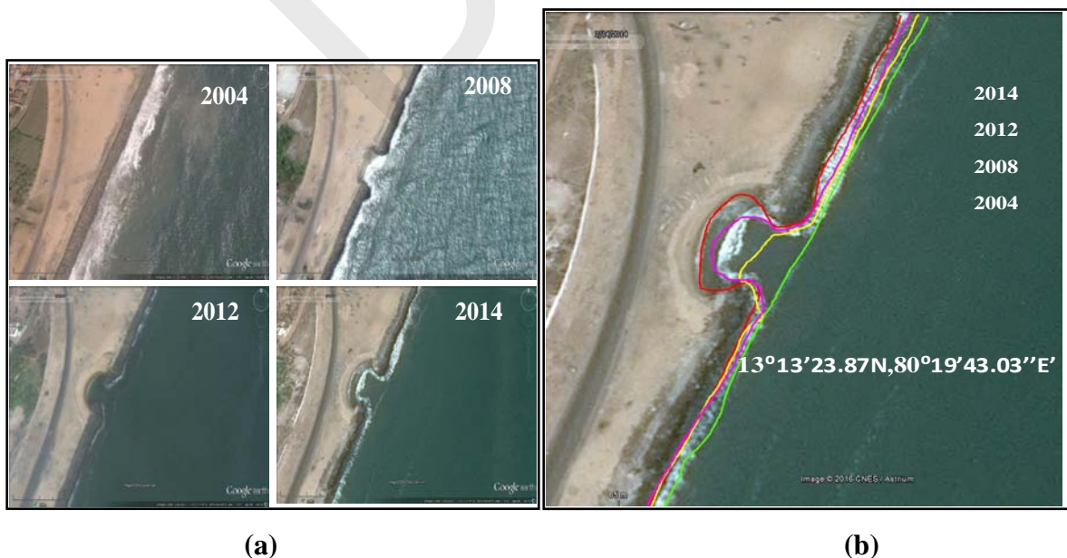
Fig. 1.31a and 1.31b Shoreline behaviour near the termination of seawalls
