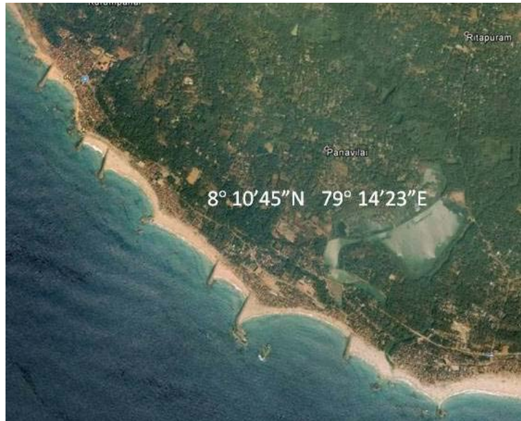
Fig.1.20. Groins field protecting the West coast of Tamilnadu
