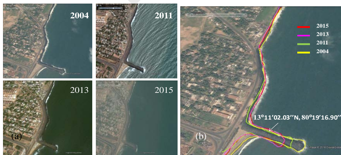
Fig. 1. 33a and 1. 33b. Behaviour of shoreline due to groin field off Chennai coast
