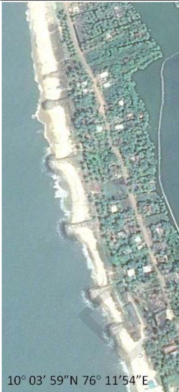
Fig.1.21. T-Gorin field protecting the coast of Narayanambalam, Kerala
