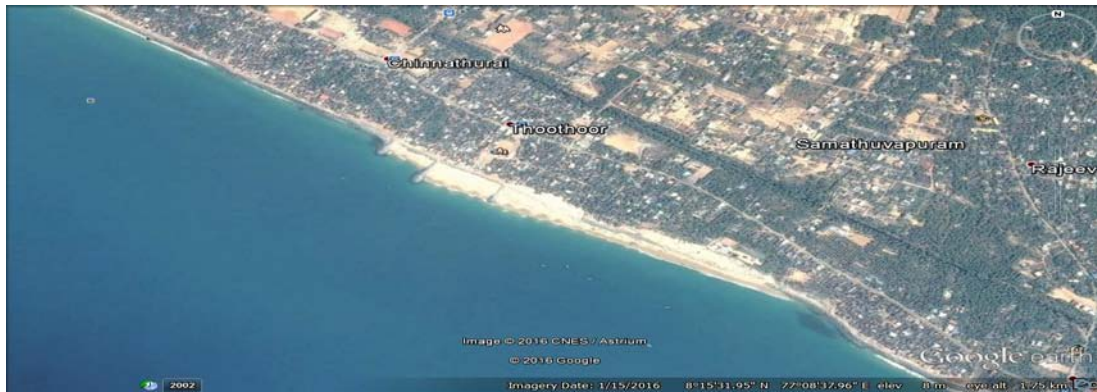
Fig.10.27a Google image showing the effectiveness of the groins at Thoothoor
