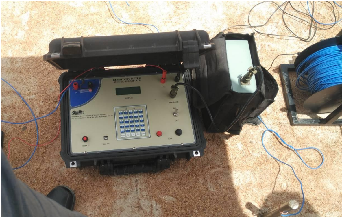
FIGURE 4 (A): VERTICAL ELECTRODE SOUNDING INSTRUMENT
