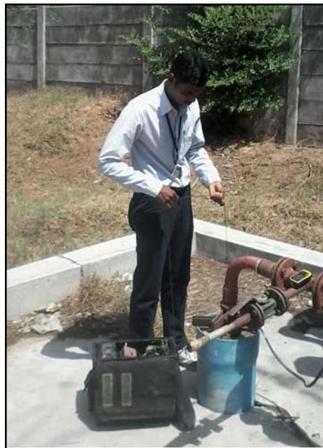
Plate 2.2: Photographs show measurement of water level with Water level indicator
