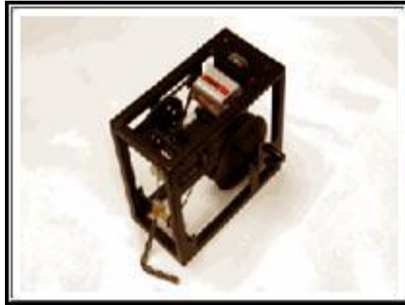
Plate 2.1: Photographs show Water Level Indicator
