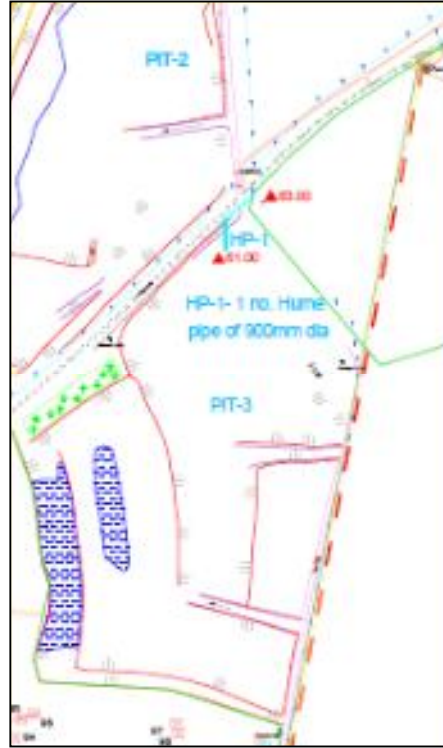
Figure-2 Hume pipe details from catchment to Pit-3.
