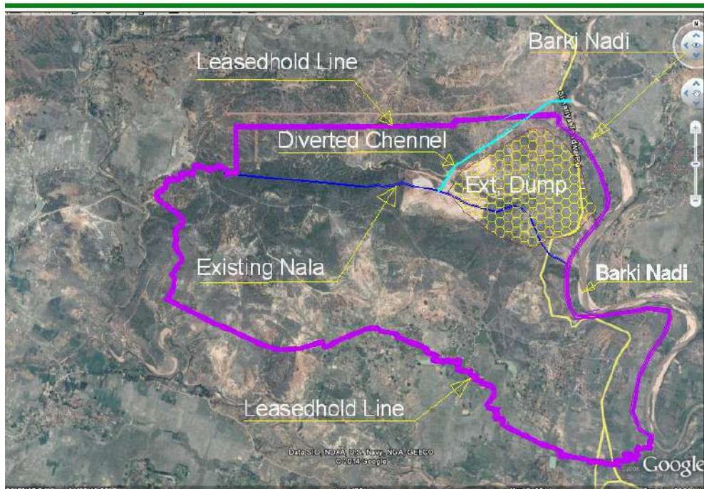
Fig: Proposed Alignment of Diverted Channel
