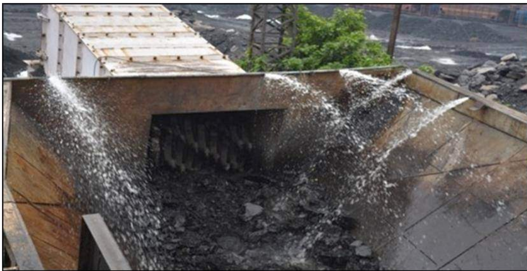
Fig: Dust Suppression at Crusher Unit
