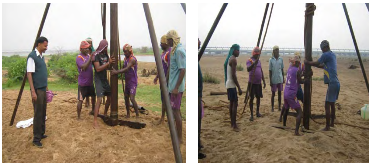
FIGURE : 4.14 Photographs showing bore log test in river bed
