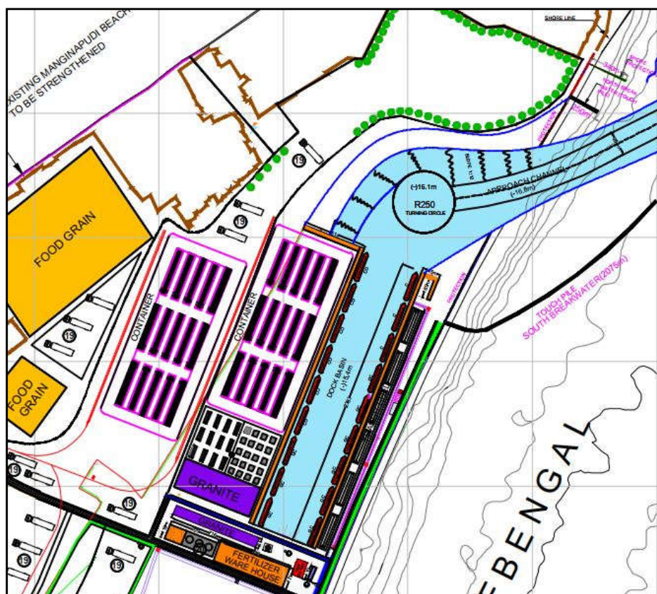
Fig 3.5: Proposed Harbour layout at Manginapudi location - basin and berths are inside the shore
