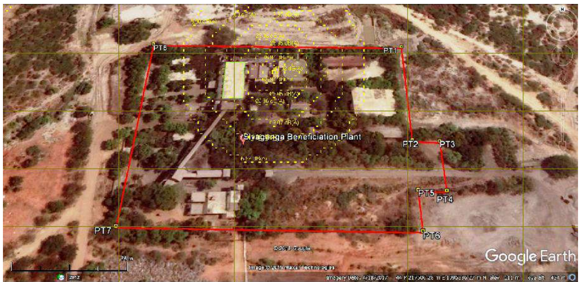
Figure 3-11 Noise contours due to DG Set 380 kVA at beneficiation plant
