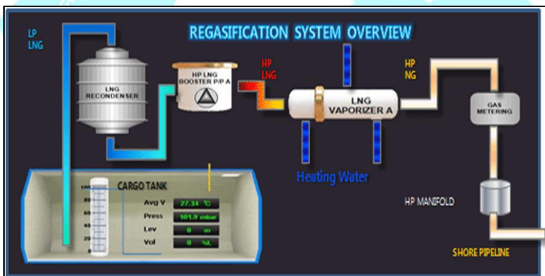
Figure 2.6: Typical FSRU Regasification System Overview
