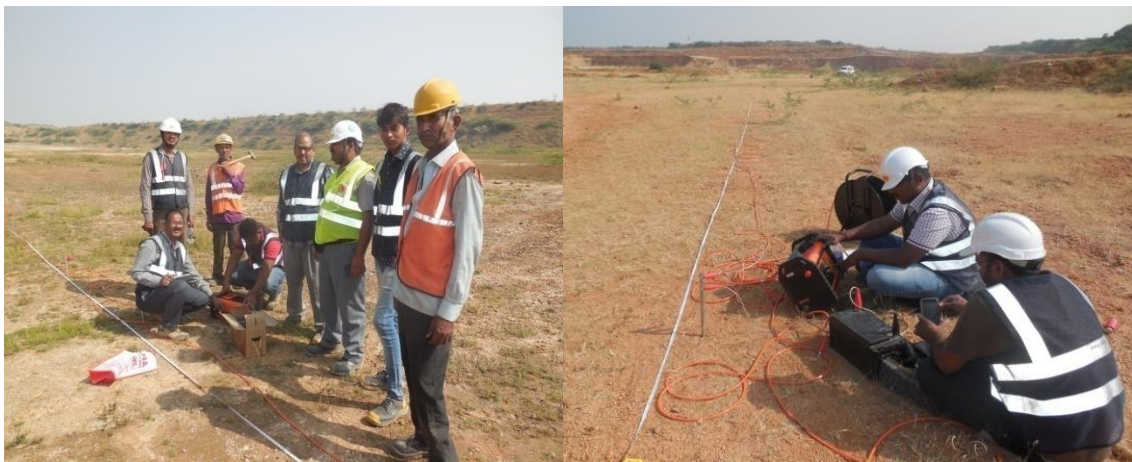
Fig. 3.9 : A field study picture of resistivity imaging survey at NCJW study area
