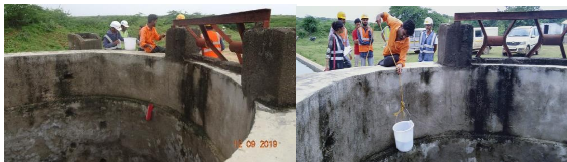
Figure 12. Observation well water sample collected from Well-5 near Varahswaroop road (Adjacent to PZM-5) during site visit of CSIR-CSMCRI
