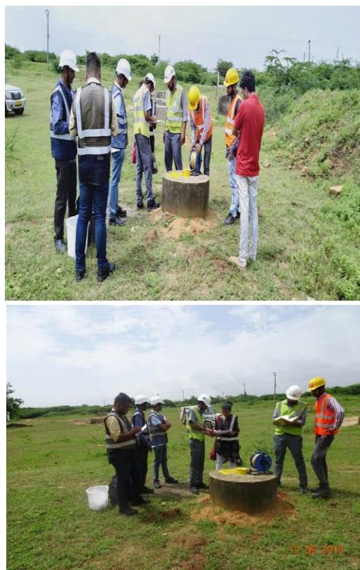
Figure 9. Piezometer head Measurement (PZM-5) near Varahswaroop road well by CSIR-CSMCRI
