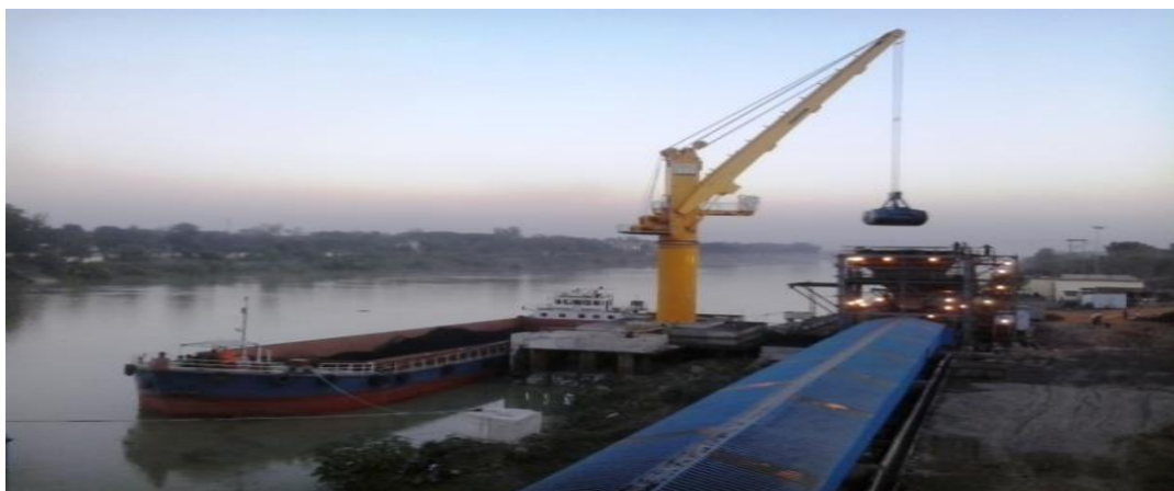
Fig. 20. Coal being unloaded from barge and loaded on to the conveyer system
