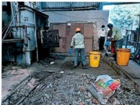
Pic. 1: Feeding of BMW through inspection door of incinerator
