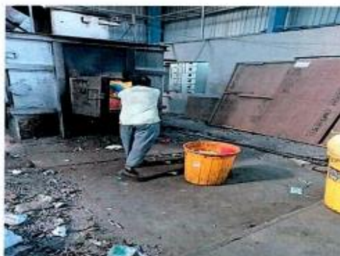
Pic. 2: Feeding of BMW through inspection door of incinerator
