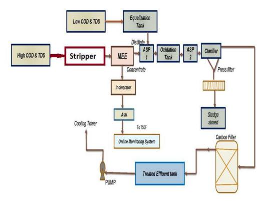
The MEE system shall be installed in the unit:
