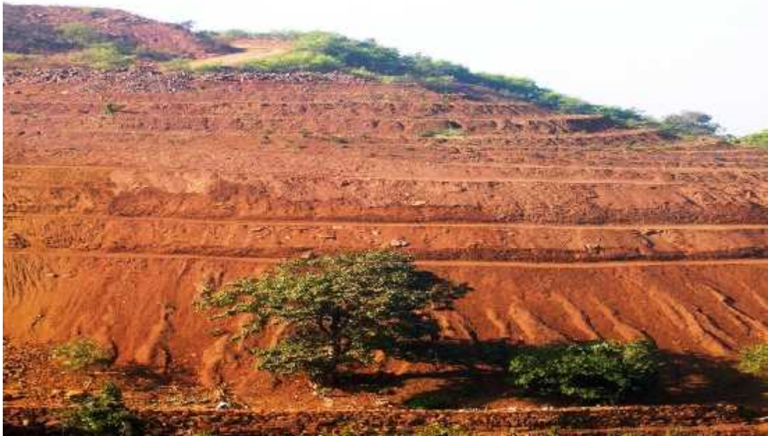
DUMP TERRACING AT N-INCLINE QUARRY
