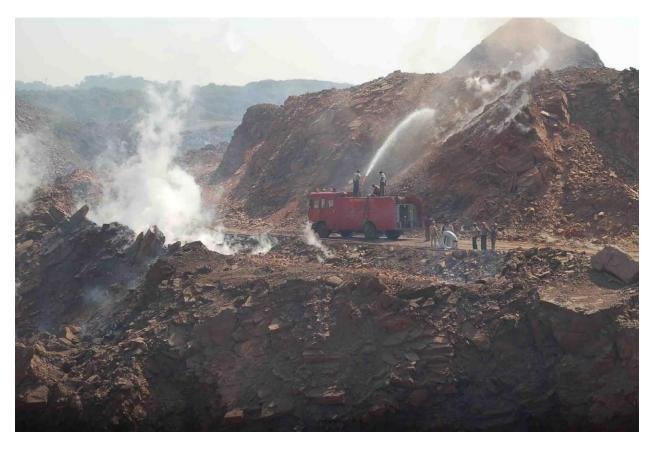
Figure 12: Quenching of coal mine fire at Rajapur fire area.
