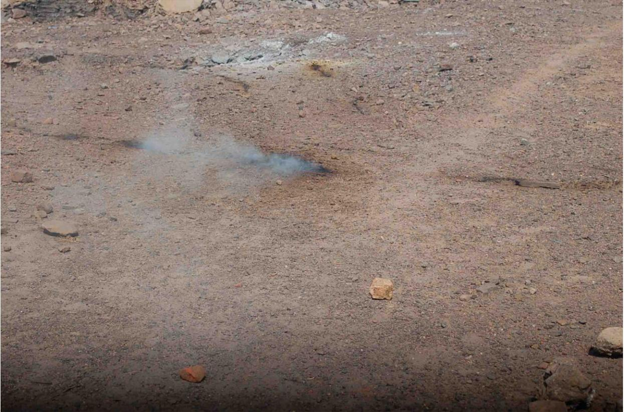
Figure 13: Cracks developed due to coal mine fire at Ghanoodih fire area.
