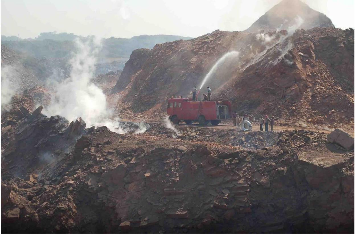
Figure 12: Quenching of coal mine fire at Rajapur fire area.
