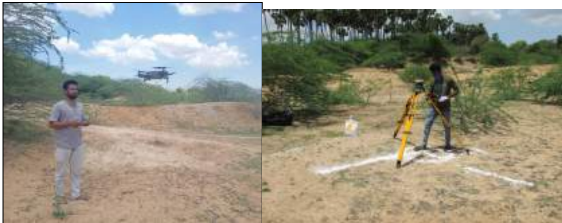
Fig.3. 2 DGPS survey for Ground control Points (GCP) and Drone for Aerial surveying
