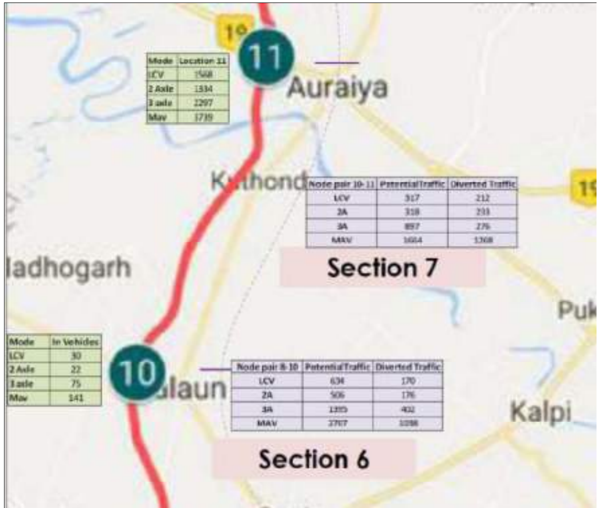
Figure 2: Potential and Diverted Traffic Assignment on to the Project Corridor between Two Nodes
