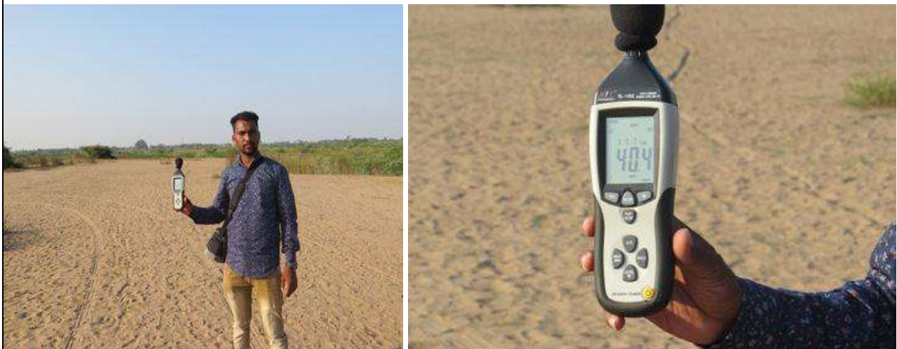
Fig.8: Image showing Measuring Noise Level
