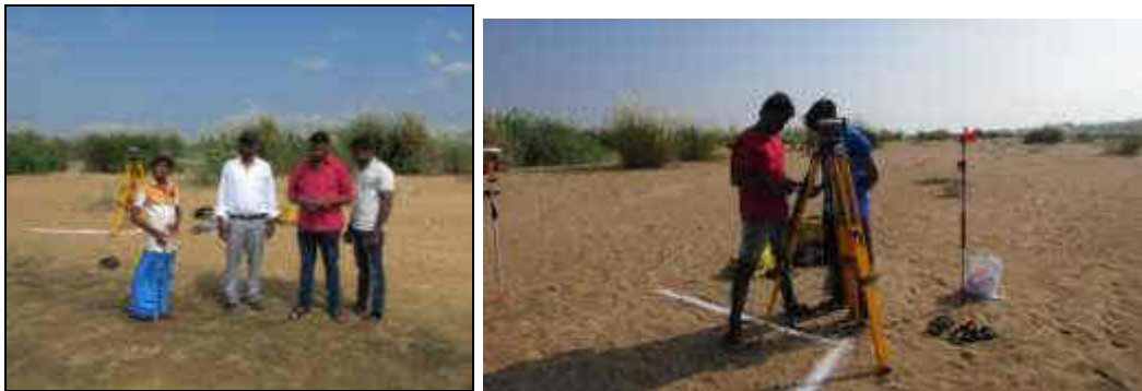
Fig.3. 2 DGPS survey for Ground control Points (GCP) and Drone for Aerial surveying
