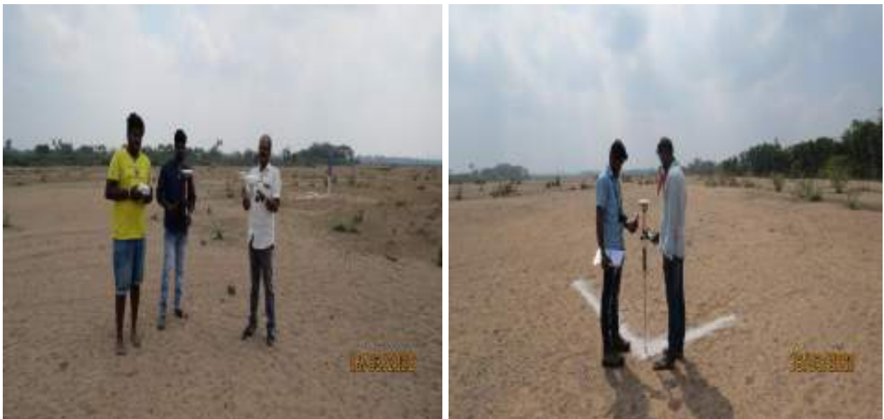
Fig:1. DGPS survey for Ground control Points (GCP) and Drone for Aerial
