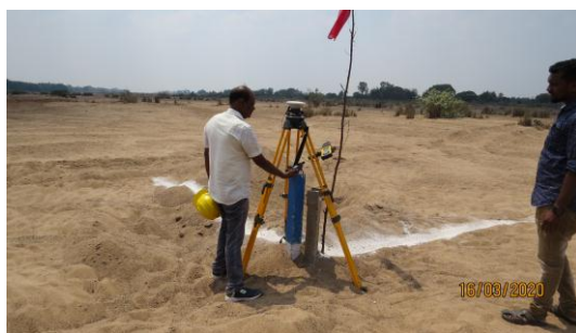
Fig. 2 DGPS survey for Pillar Points (PP) and Drone for Aerial surveying
