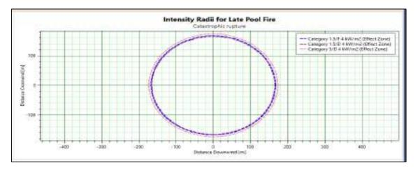
Late Explosion worst case radii in case of Catastrophic Rupture of Formaldehyde Storage Tank
