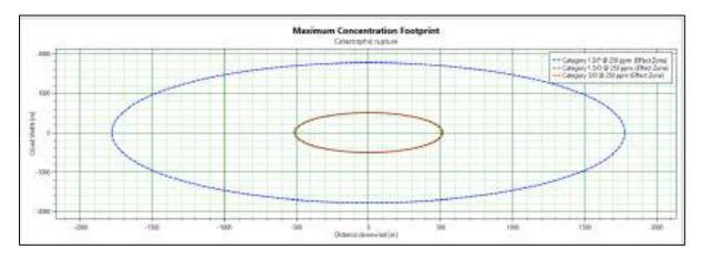
Maximum Concentration footprint in case of catastrophic rupture of methanol Storage Tank
