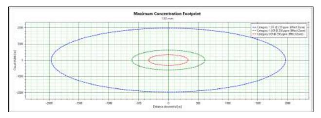
Maximum Concentration Footprint envelope in case 100mm leak of Methanol Storage Tank
