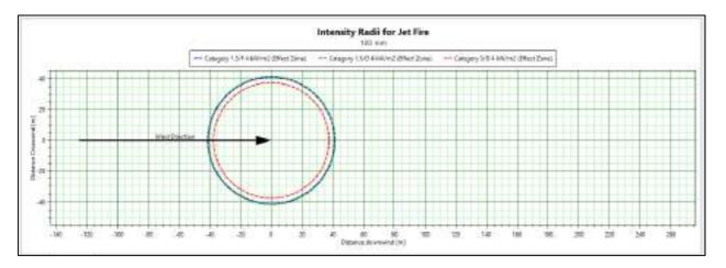
Jet Fire envelope Intensity radii in case of 100mm leak of Methanol Storage Tank
