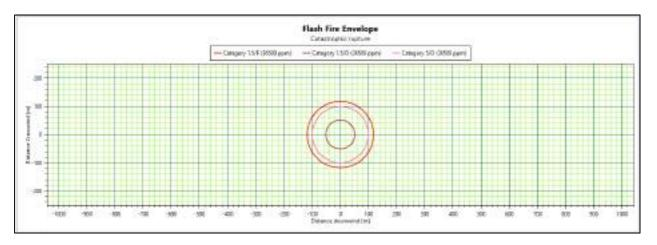
Flash Fire envelope in case of catastrophic rupture of Methanol Storage Tank
