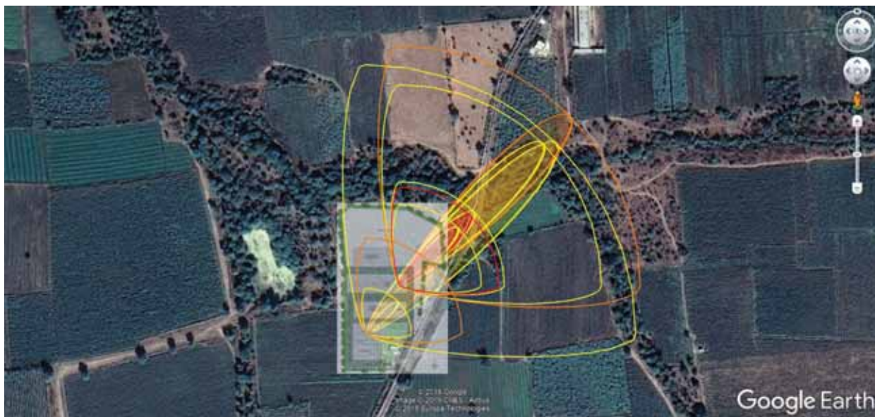
Figure 7.4: Toxic threat zone of all the chemicals considered
