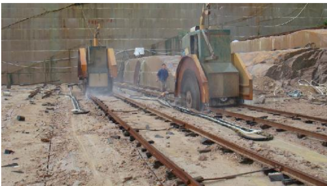
Fig.7.8: Face cutting equipments with gang saw blade using rail tracks alignment
