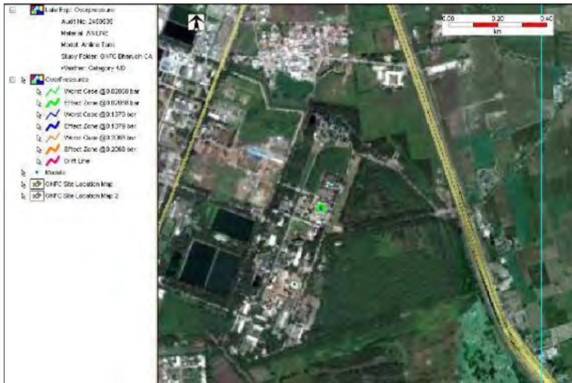
Figure 7-5: Late Explosion overpressure risk contour catastrophic rupture of Aniline tank at 4.0/D
