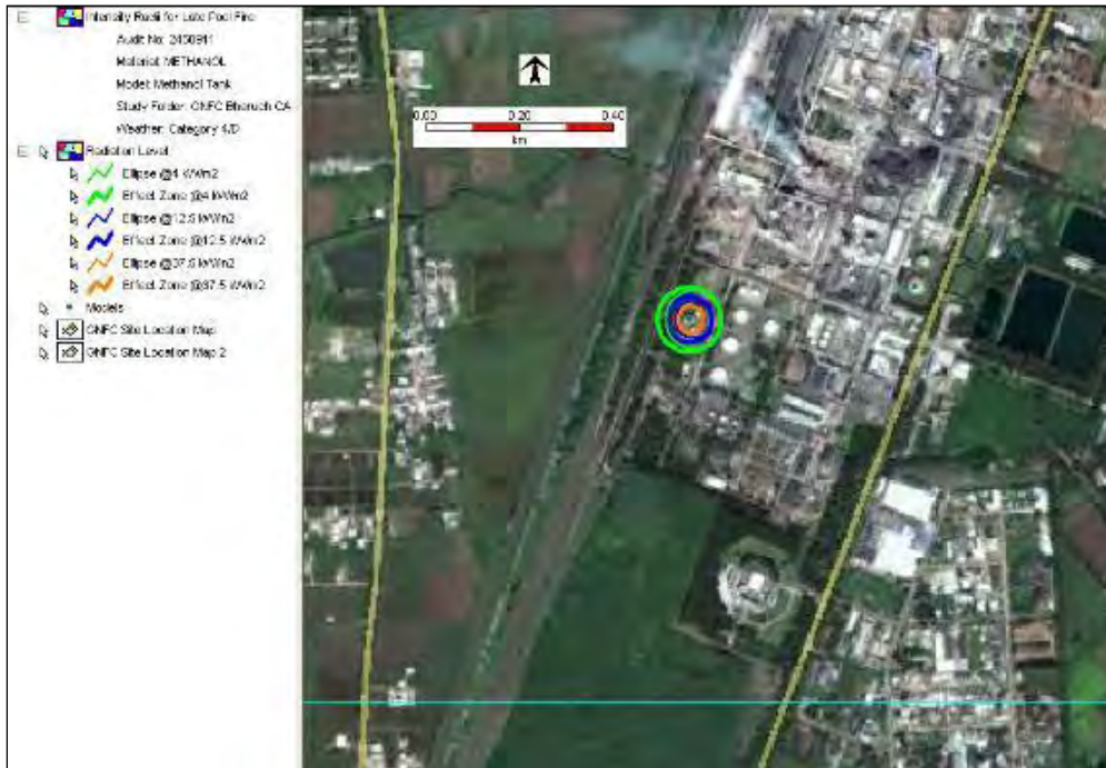
Figure 7-9: Late pool fire risk contour - Catastrophic Rupture in Methanol tank at 4.0/D
