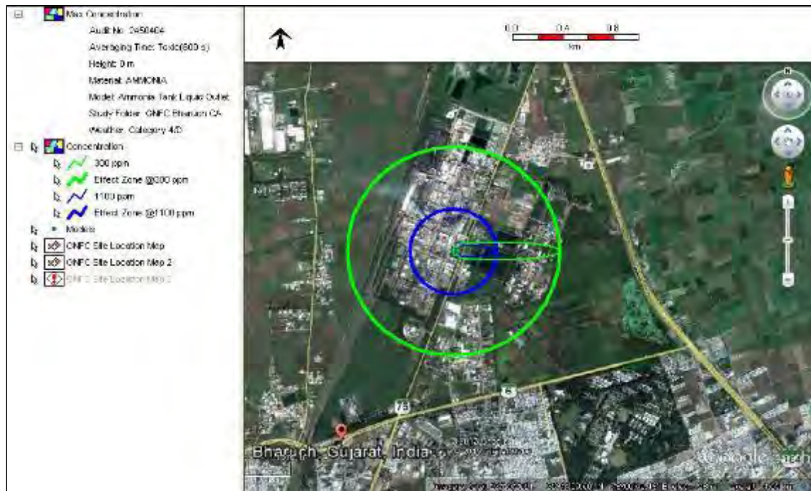
Figure 7-2: Late pool fire risk contour due to 50 mm Leak in Ammonia tank at weather 4.0/D
