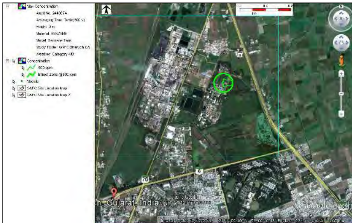
Figure 7-8: Concentration risk contour - Catastrophic Rupture of Benzene tank at 4.0/D
