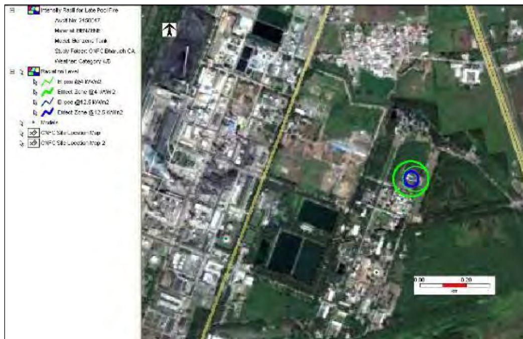
Figure 7-6: Late pool fire risk contour - Catastrophic Rupture in Benzene tank at 4.0/D
