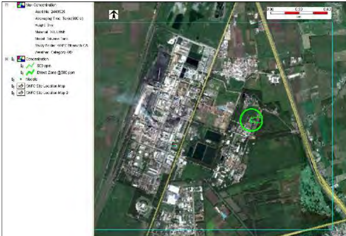
Figure 7-15: Concentration risk contour - Catastrophic Rupture of Toluene tank at 4.0/D
