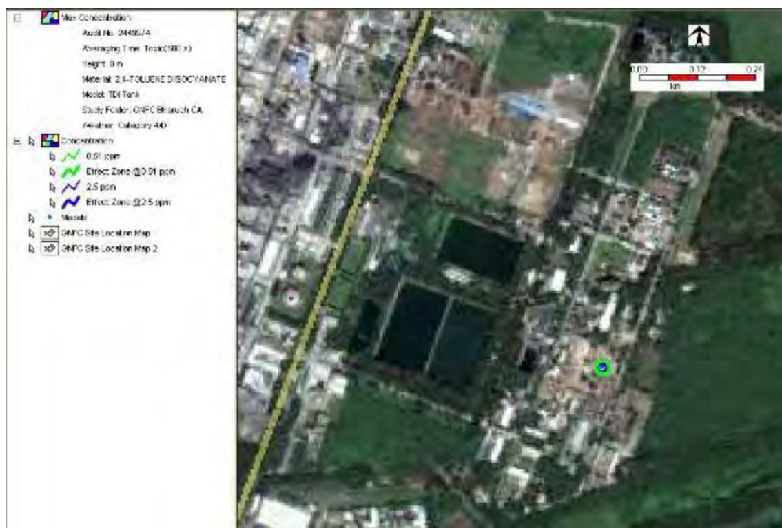
Figure 7-16: Concentration risk contour - Catastrophic Rupture of TDI tank at 4.0/D
