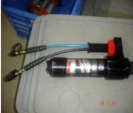
Ram Jack- used to create gap of ~575 cm stroke
