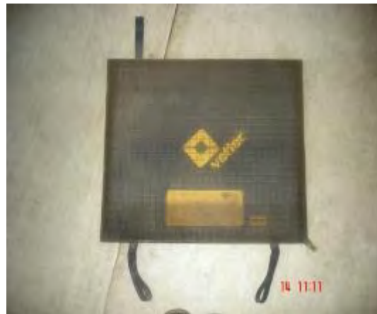
Lifting Bag- To lift 68 ton load up to 52 cm height
