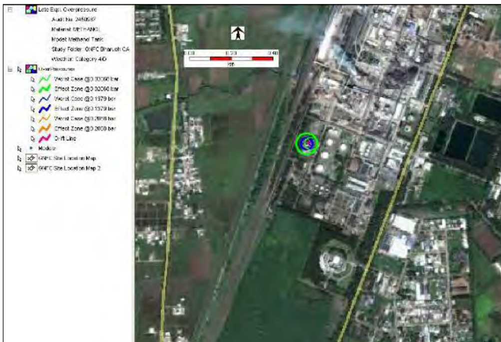
Figure 7-10: Late Explosion overpressure risk contour - Catastrophic rupture of Methanol tank at 4.0/D
