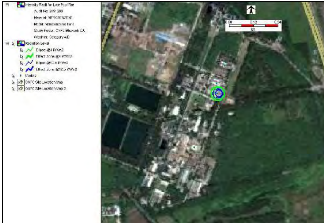
Figure 7-12: Late Explosion overpressure risk contour - Catastrophic rupture of Nitrobenzene tank at 4.0/D
