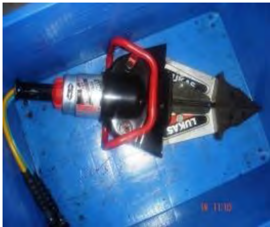
Spreader- To create gap up to 720 mm distance
