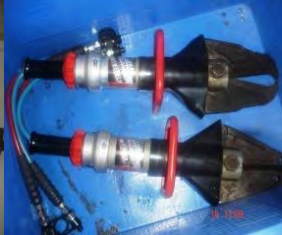
Cutter- Used for cutting up to 30 mm round steel diameter
