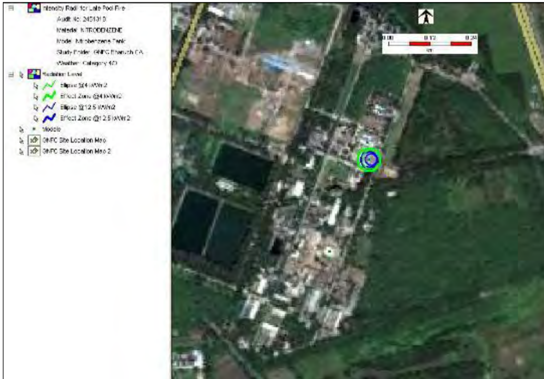
Figure 7-11: Late pool fire risk contour - Catastrophic Rupture in Nitrobenzene tank at 4.0/D
