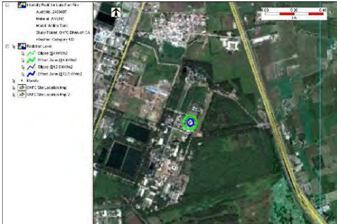
Figure 7-4: Late pool fire risk contour - Catastrophic Rupture in Aniline tank at 4.0/D
