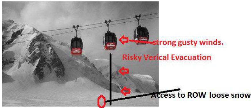
Figure 7.6: Impact of strong gusty wind, Risky during ropeway stuck-up due to Mechanical Failure
