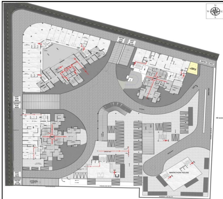
Fig. 6.8 Ground floor evacuation layout
