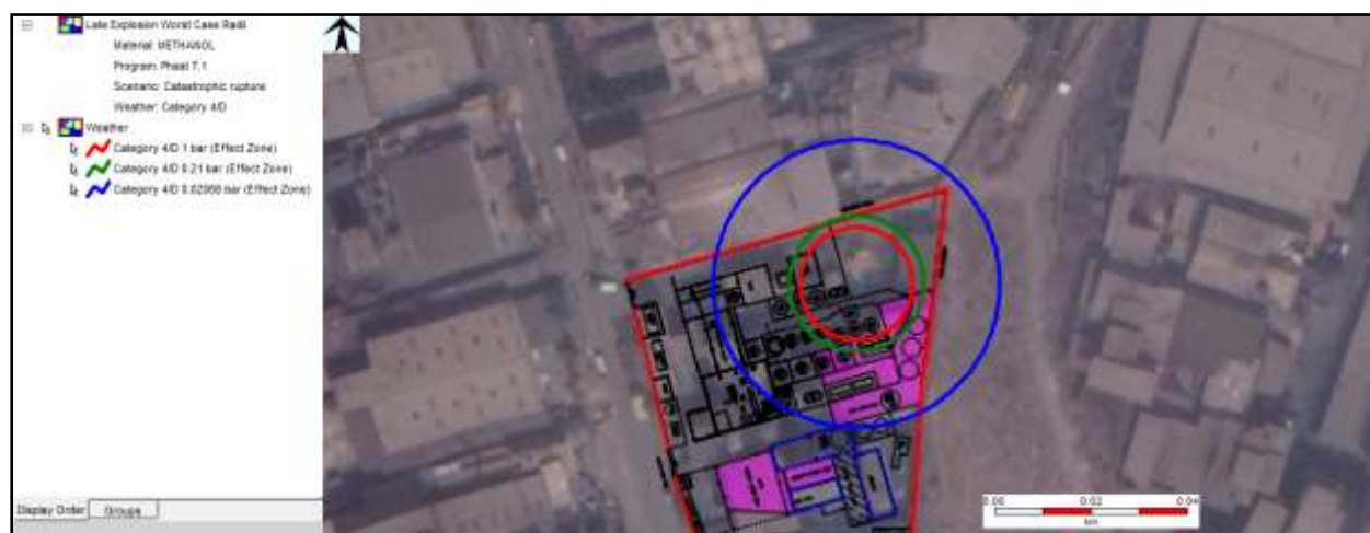
Figure 7-13: Overpressure effect Consequence Contour due to Catastrophic Rupture at Weather Condition 4.0/D
