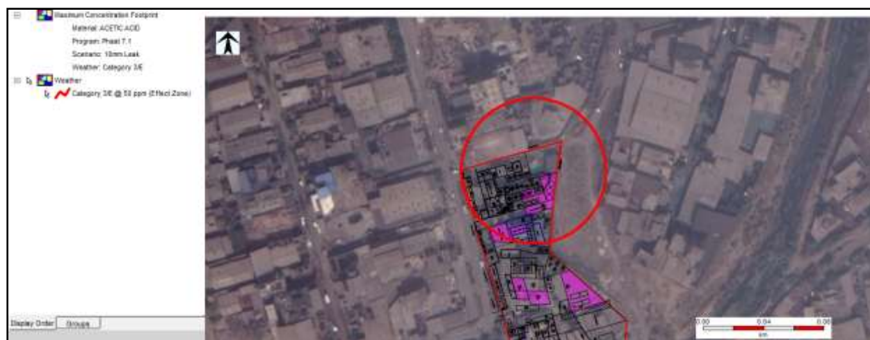
Figure 7-4: Maximum Concentration effect Consequence Contour due to 10 mm hole leak at Weather Condition 3.0/E
