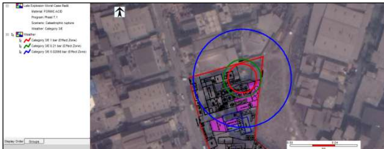
Figure 7-15: Toxic Consequence Contour due to Catastrophic Rupture at Weather Condition 3.0/E
