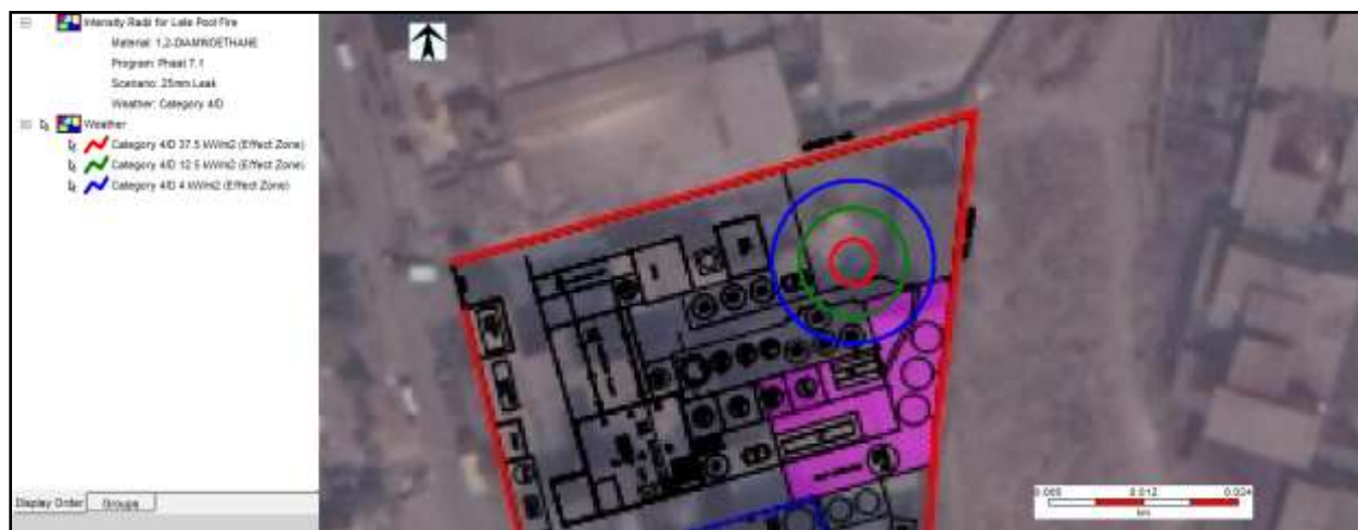
Figure 7-10: Overpressure effect Consequence Contour due to Catastrophic Rupture at Weather Condition 3.0/E
