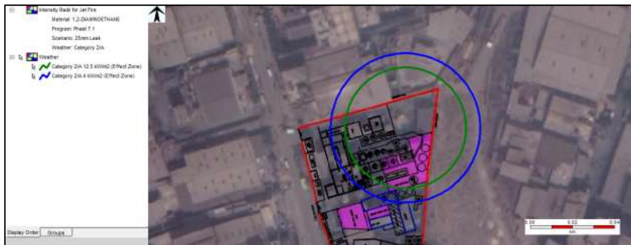
Figure 7-9: Late Pool Fire effect Consequence Contour due to 25 mm leak at Weather Condition 4.0/D
