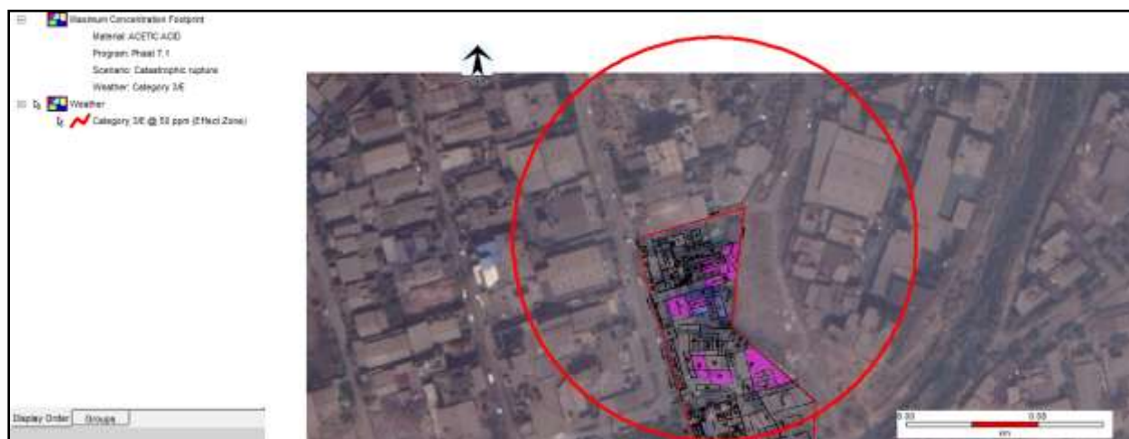
Figure 7-5: Maximum Concentration effect Consequence Contour due to Catastrophic Rupture at Weather Condition 3.0/E
