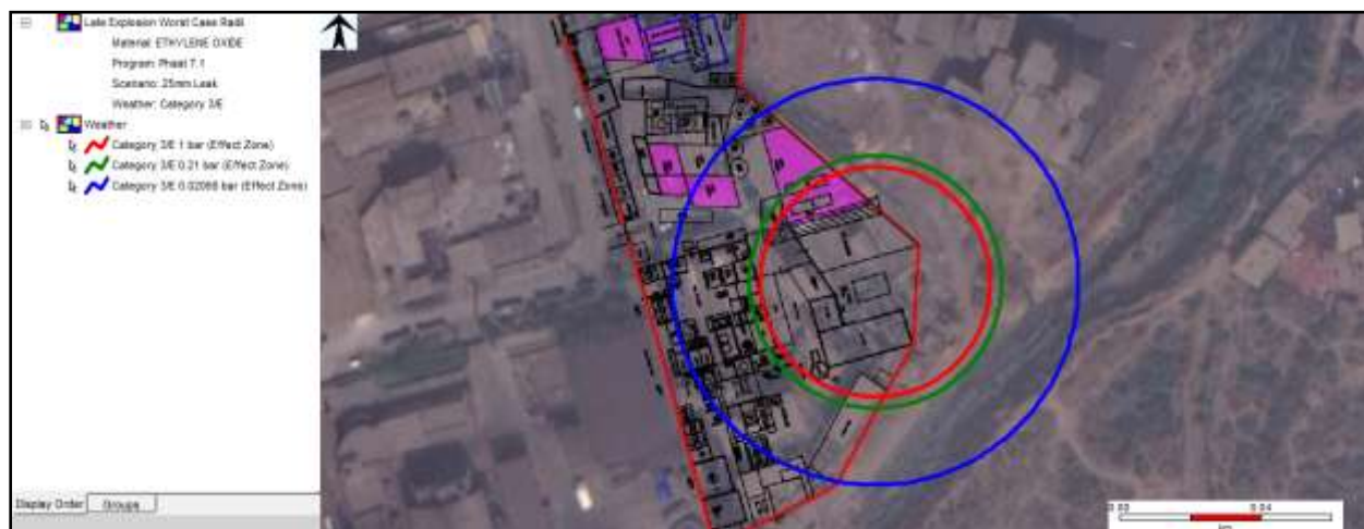
Figure 7-3: Overpressure effect Consequence Contour due to 25 mm hole leak at Weather Condition 3.0/E
