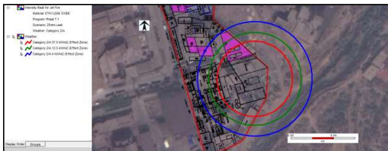
Figure 7-1: Jet Fire effect Consequence Contour due to 25 mm hole leak at Weather Condition 2.0/A
