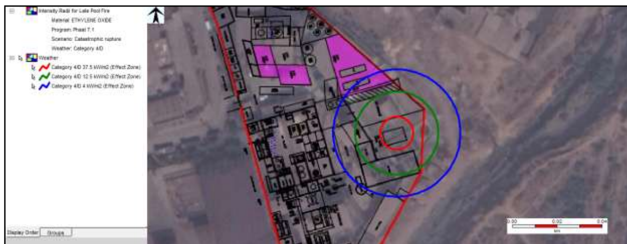
Figure 7-3: Overpressure effect Consequence Contour due to 25 mm hole leak at Weather Condition 3.0/E
