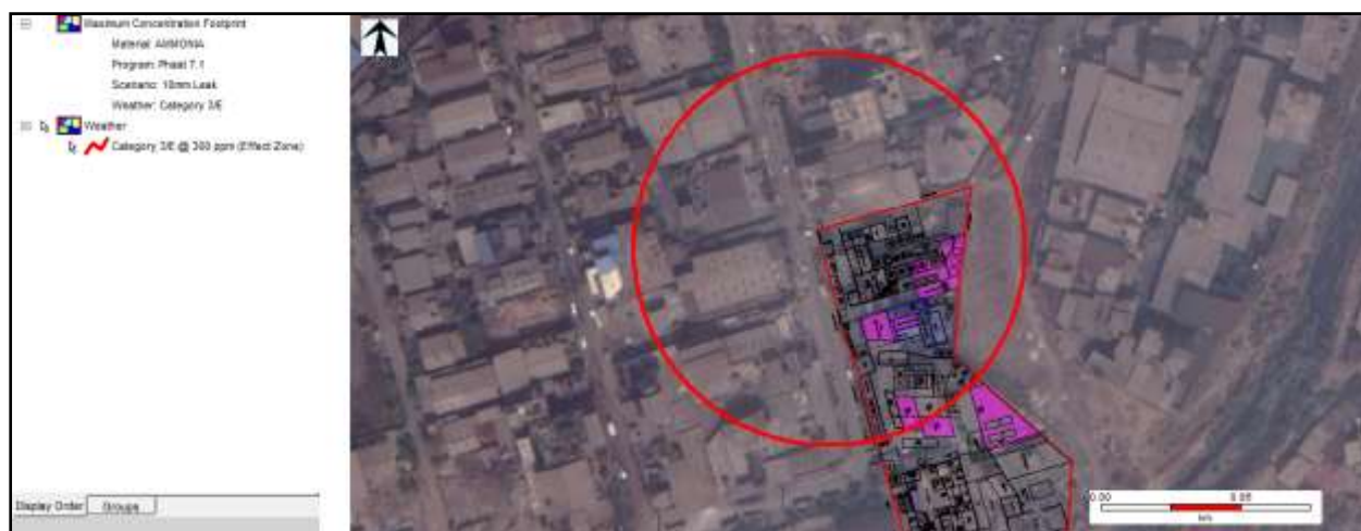
Figure 7-6: Toxic Consequence Contour due to 10 mm hole leak at Weather Condition 3.0/E
