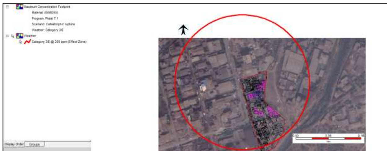
Figure 7-7: Toxic Consequence Contour due to Catastrophic Rupture at Weather Condition 3.0/E
