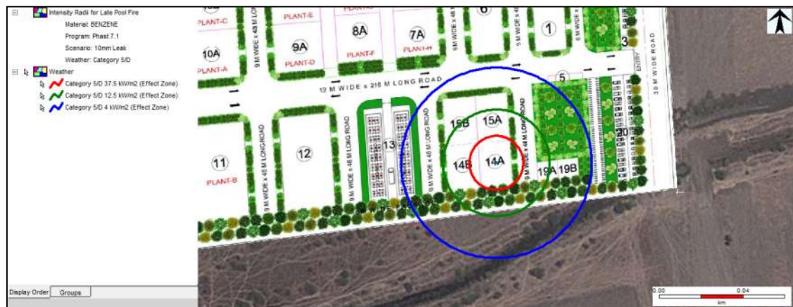
Figure 7-6: Late Pool Fire Risk Consequence Contour due to 10 mm leak in Benzene Storage Tank at Weather Condition 5.0/D
