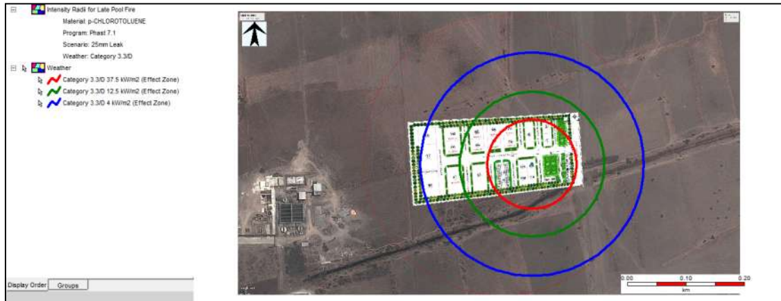
Figure 7-23: Late Explosion Risk Consequence Contour of p-Chloro Toluene due to Catastrophic Rupture at Weather Condition 3.3/D
