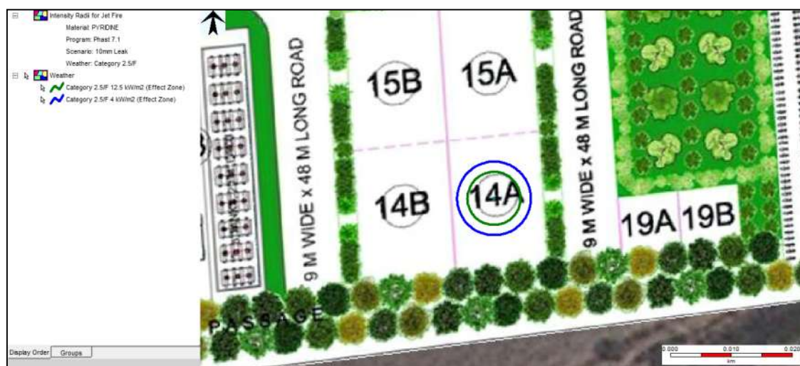
Figure 7-31: Jet Fire Risk Consequence Contour of Pyridine due to 25 mm leak at Weather Condition 3.3/D
