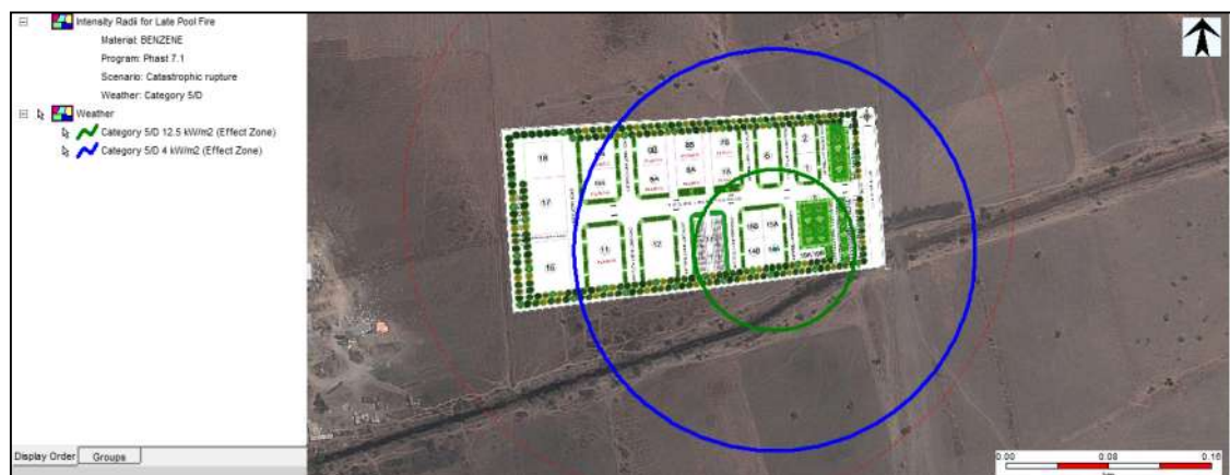
Figure 7-9: Late Explosion Risk Consequence Contour due to Catastrophic Rupture of Benzene Storage Tank at Weather Condition 5.0/D
