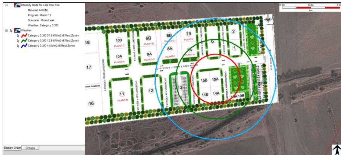
Figure 7-2: Toxic Effect Contour due to 10 mm leak in Aniline Storage Tank at Weather Condition 2.5/F
