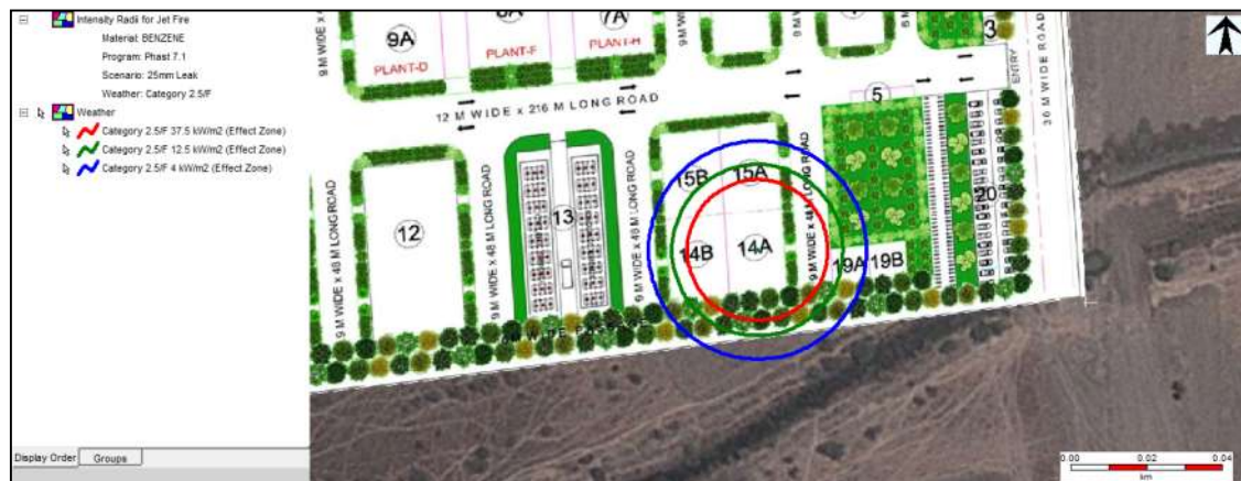
Figure 7-9: Late Explosion Risk Consequence Contour due to Catastrophic Rupture of Benzene Storage Tank at Weather Condition 5.0/D
