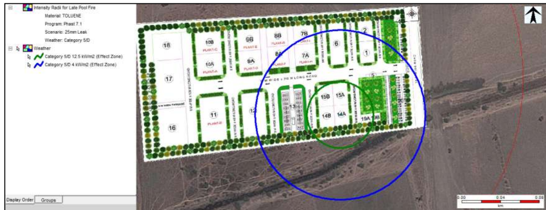
Figure 7-35: Late Explosion Risk Consequence Contour of Toluene due to Catastrophic Rupture at Weather Condition 2.5/F
