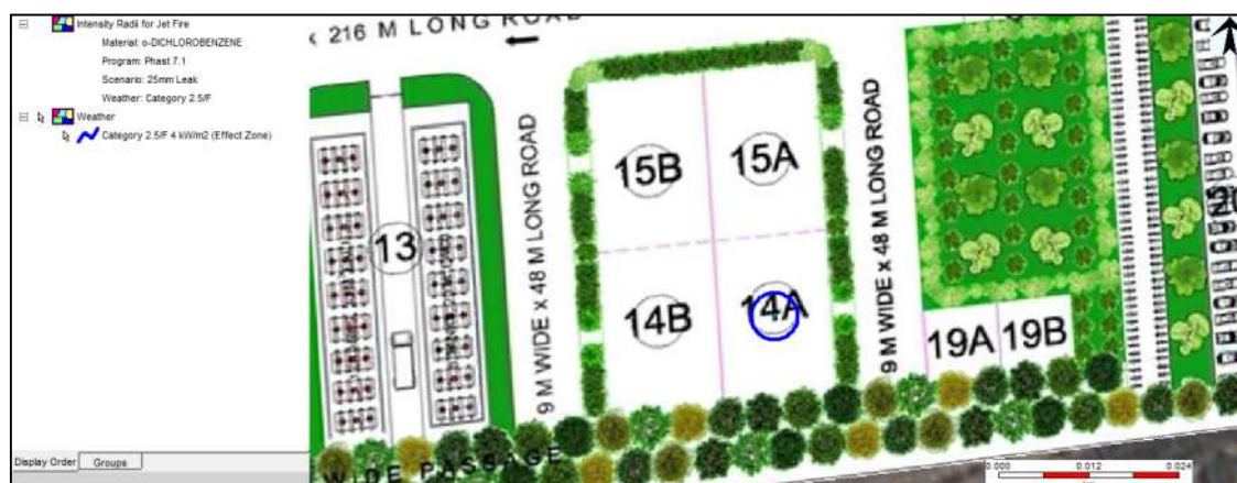
Figure 7-18: Jet Fire Risk Consequence Contour of ODCB due to 25mm leak at Weather Condition 2.5/F
