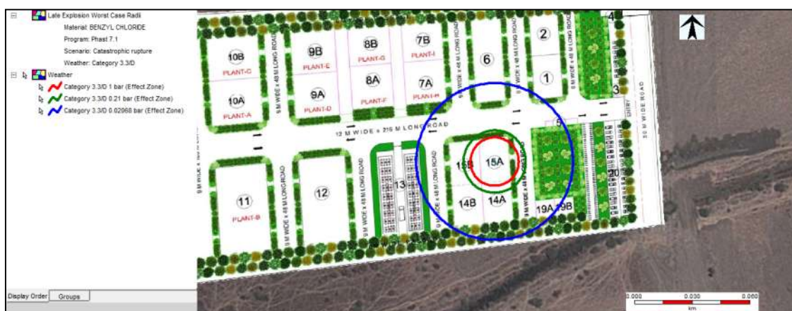
Figure 7-13: Toxic Effect Contour of Benzyl Chloride due to 10 mm leak at Weather Condition 2.5/f
