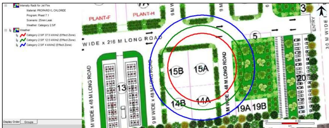
Figure 7-29: Late Explosion Risk Consequence Contour of Propargyl Chloride due to 10 mm leak at Weather Condition 2.5/F
