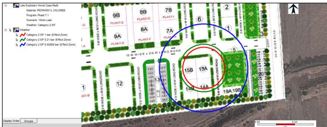
Figure 7-29: Late Explosion Risk Consequence Contour of Propargyl Chloride due to 10 mm leak at Weather Condition 2.5/F
