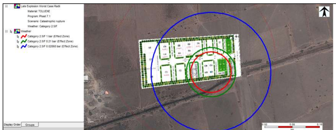
Figure 7-35: Late Explosion Risk Consequence Contour of Toluene due to Catastrophic Rupture at Weather Condition 2.5/F
