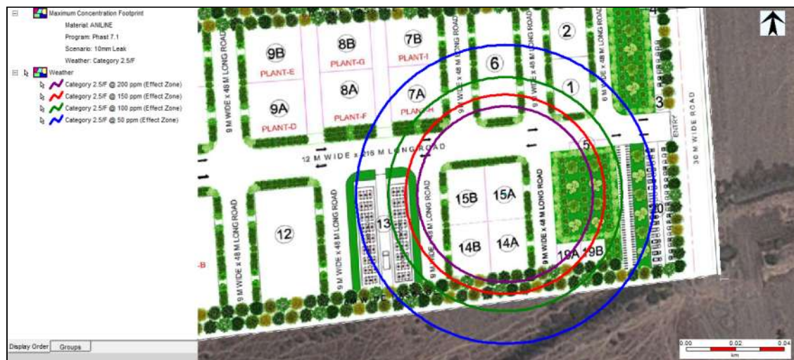
Figure 7-2: Toxic Effect Contour due to 10 mm leak in Aniline Storage Tank at Weather Condition 2.5/F
