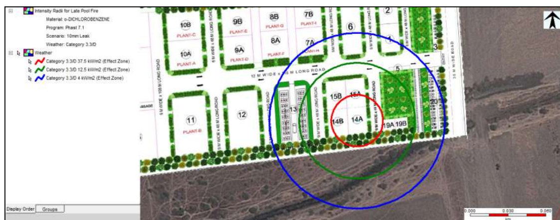
Figure 7-18: Jet Fire Risk Consequence Contour of ODCB due to 25mm leak at Weather Condition 2.5/F
