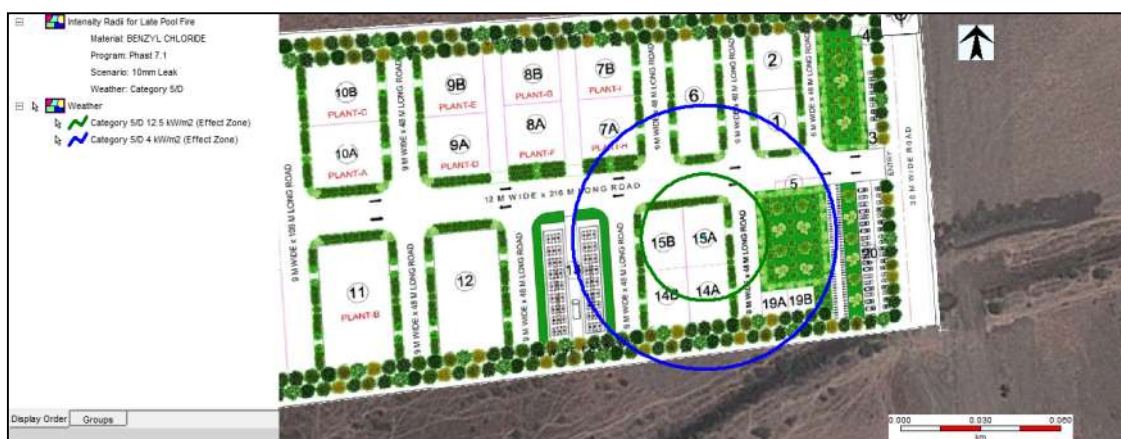
Figure 7-11: Late Pool Fire Risk Consequence Contour of Benzyl Chloride due to 10 mm leak at Weather Condition 5.0/D
