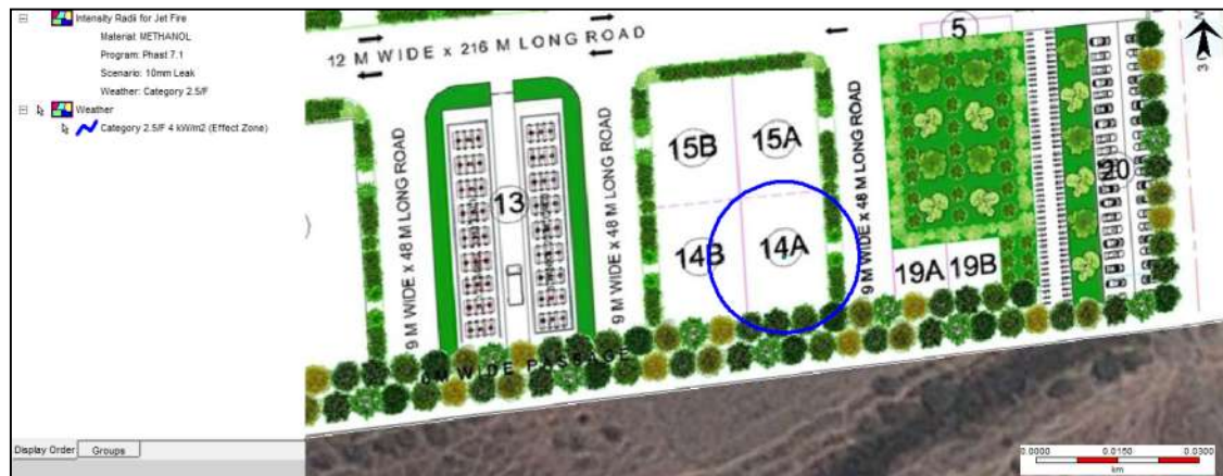
Figure 7-15: Late Pool Fire Risk Consequence Contour of Methanol due to 25 mm leak at Weather Condition 2.5/F
