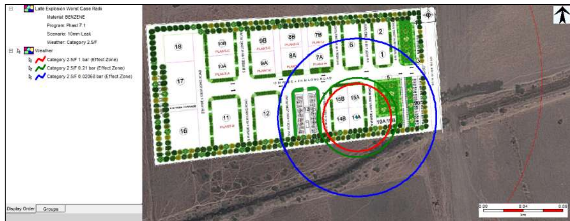
Figure 7-8: Jet Fire Risk Consequence Contour due to 25 mm leak in Benzene Storage Tank at Weather Condition 2.5/F
