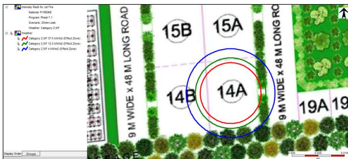
Figure 7-31: Jet Fire Risk Consequence Contour of Pyridine due to 25 mm leak at Weather Condition 3.3/D
