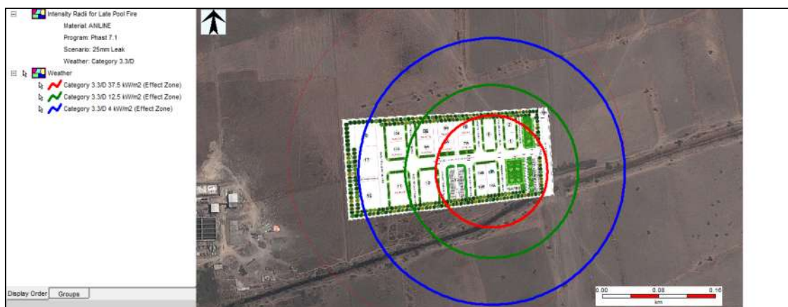
Figure 7-4: Late explosion effect contour due to 25 mm leak in Aniline storage tank at weather condition 3.3/D
