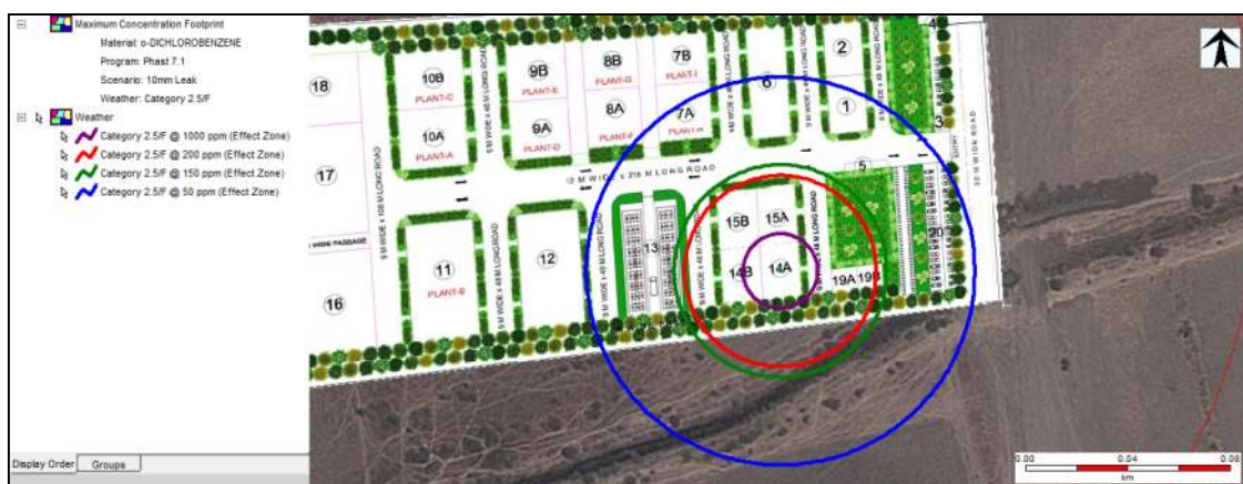
Figure 7-20: Toxic Effect Contour of ODCB due to 10 mm leak at Weather Condition 2.5/F
