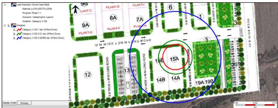
Figure 7-23: Late Explosion Risk Consequence Contour of p-Chloro Toluene due to Catastrophic Rupture at Weather Condition 3.3/D
