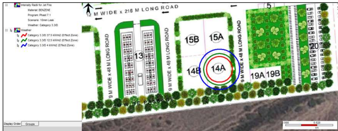
Figure 7-6: Late Pool Fire Risk Consequence Contour due to 10 mm leak in Benzene Storage Tank at Weather Condition 5.0/D
