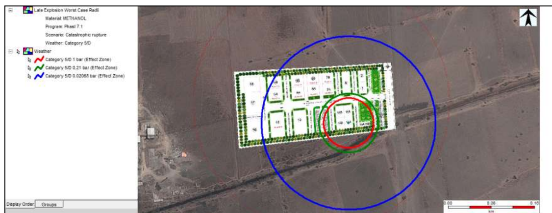
Figure 7-16: Late Explosion Risk Consequence Contour of Methanol due to Catastrophic Rupture at Weather Condition 5.0/D
