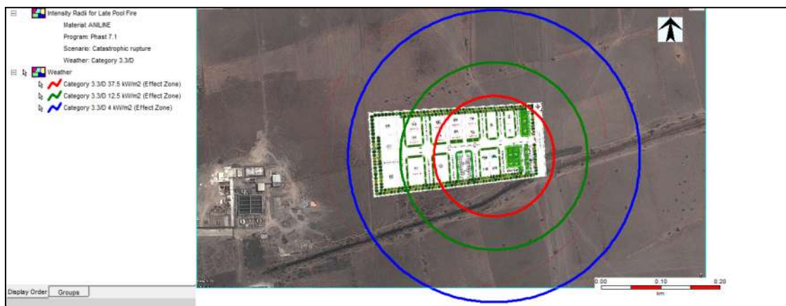
Figure 7-4: Late explosion effect contour due to 25 mm leak in Aniline storage tank at weather condition 3.3/D
