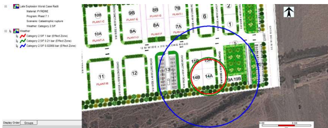
Figure 7-32: Late Explosion Risk Consequence Contour of Pyridine due to Catastrophic Rupture at Weather Condition 2.5/F
