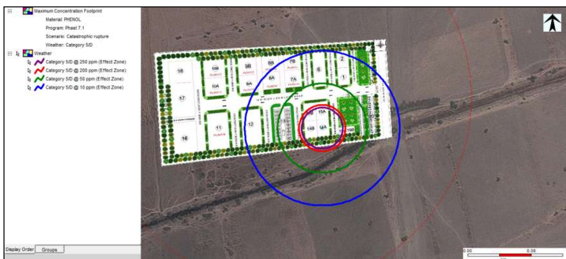
Figure 7-26: Toxic Effect Contour of Phenol due to Catastrophic Rupture at Weather Condition 5.0/D
