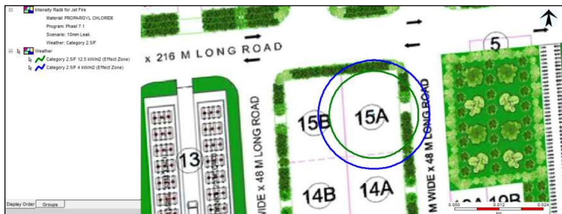
Figure 7-27: Jet Fire Risk Consequence Contour of Propargyl Chloride due to 10 mm leak at Weather Condition 2.5/F
