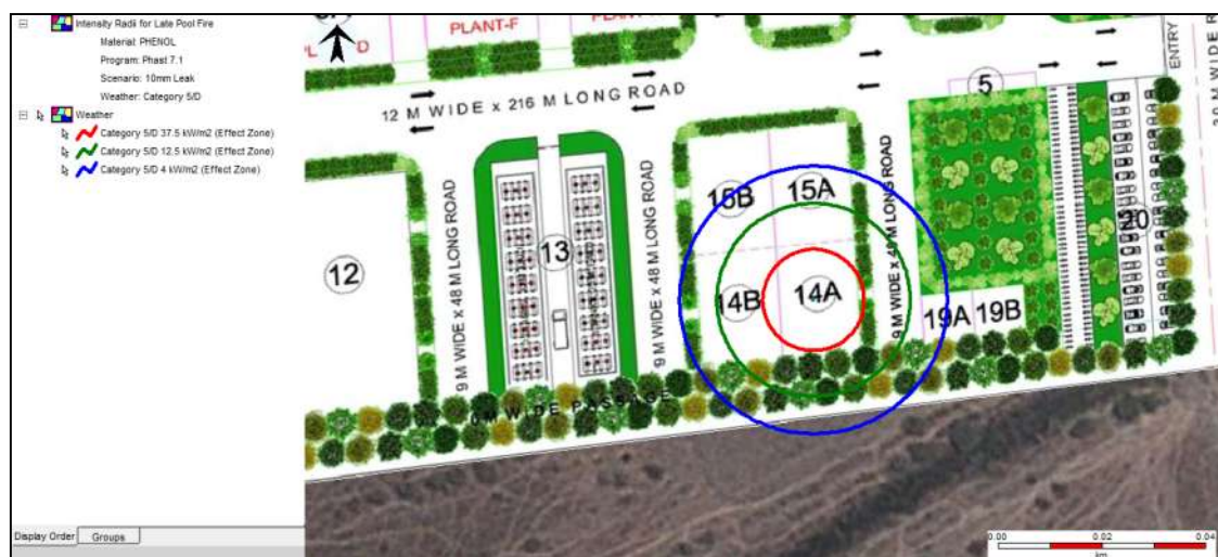
Figure 7-25: Jet Fire Risk Consequence Contour of Phenol due to 25mm leak at Weather Condition 2.5/F
