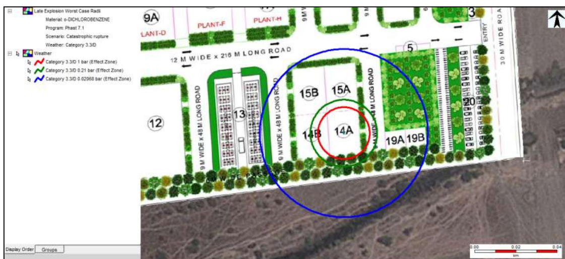
Figure 7-20: Toxic Effect Contour of ODCB due to 10 mm leak at Weather Condition 2.5/F
