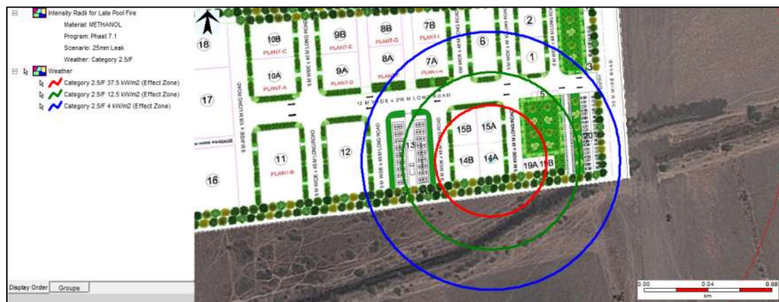
Figure 7-16: Late Explosion Risk Consequence Contour of Methanol due to Catastrophic Rupture at Weather Condition 5.0/D
