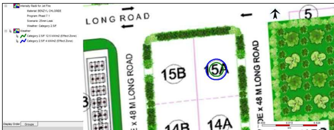
Figure 7-11: Late Pool Fire Risk Consequence Contour of Benzyl Chloride due to 10 mm leak at Weather Condition 5.0/D
