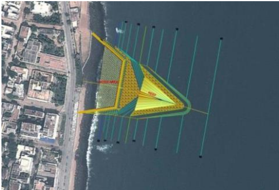
Figure 3.1 Detailed design of the wedge reef. The reef is a single concrete unit resting on a bed of rocks laid horizontally at -2.5 m. The work area is shown in the lee and the gap between the reef and work area is filled with rocks to Chart Datum level.
