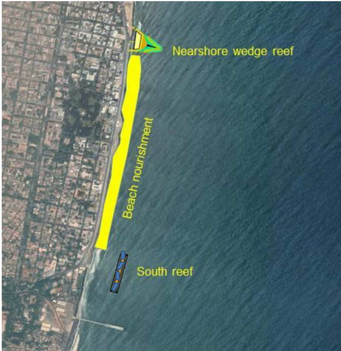
Figure 1.1 Puducherry beach restoration interventions - beach nourishment using 450,000 m 3 of sand, nearshore wedge reef in the north which acts as a sand retention structure as well as allowing sand bypassing to the north and an offshore reef at the south at 300 m north of the new pier groyne to increase the longevity of the beach nourishment.
