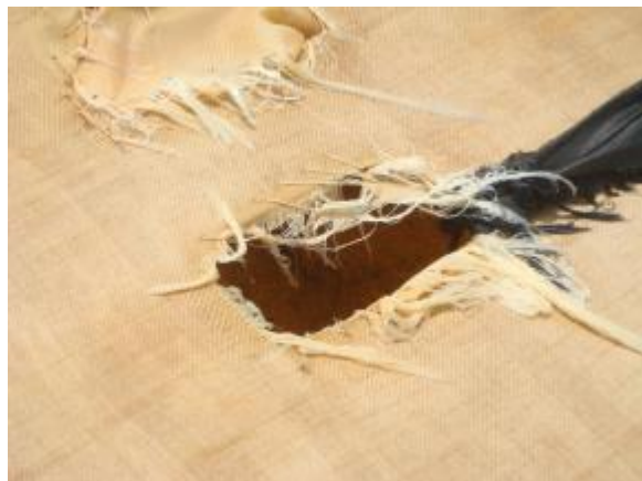
Figure 3.31 Punctured woven geotextile - Candolim, Goa
