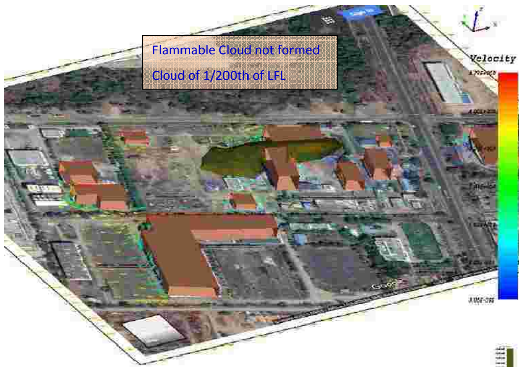
Figure 14: 3D Cloud of 5.0E-05 volume fraction, Scenario [5D-285°]
