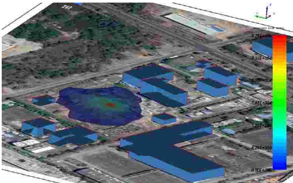
Figure 23: Impact area (no threat zone identified) of 37.5KW/m 2 Heat Radiation
