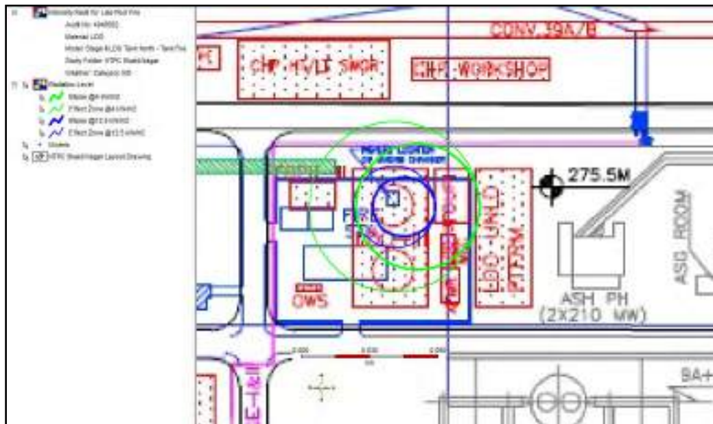
FIGURE-8 STAGE-III LDO TANK (NORTH) – TANK SURFACE FIRE
