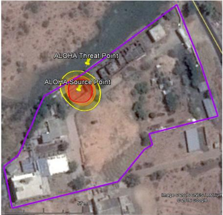
greater than 10.0 kW/(sq m) (potentially lethal within 60 sec) greater than 5.0 kW/(sq m) (2nd degree burns within 60 sec) greater than 2.0 kW/(sq m) (pain within 60 sec)
