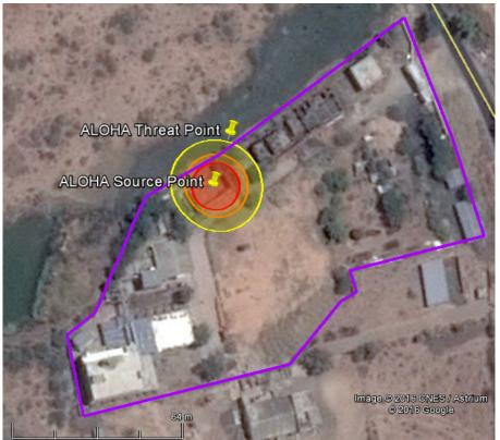
greater than 10.0 kW/(sq m) (potentially lethal within 60 sec) greater than 5.0 kW/(sq m) (2nd degree burns within 60 sec) greater than 2.0 kW/(sq m) (pain within 60 sec)
