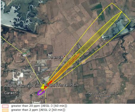
greater than 0.5 ppm (AEGL-1 [60 min]) - wind direction confidence lines
