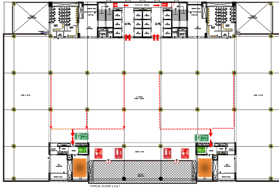
Figure 1.6 Evacuation Plan_ Typical floor plan 1, 3 & 7 floor
