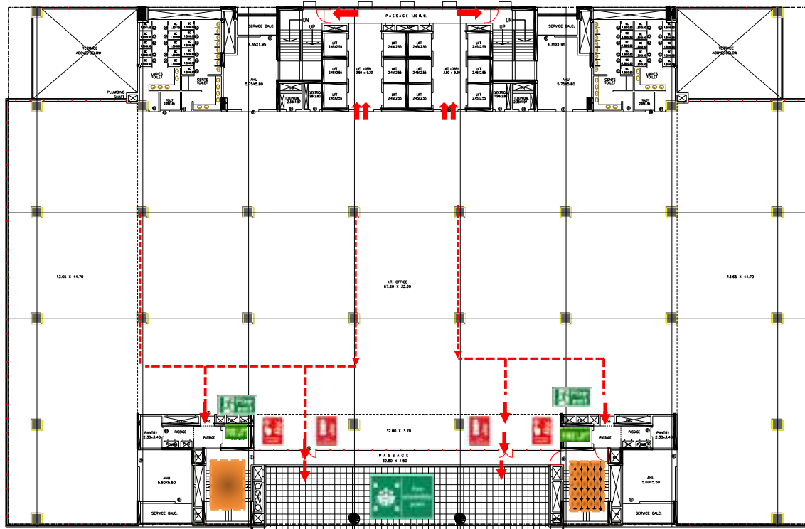
Figure 1.8 Evacuation Plan _Refuge floor plan 9th floor
