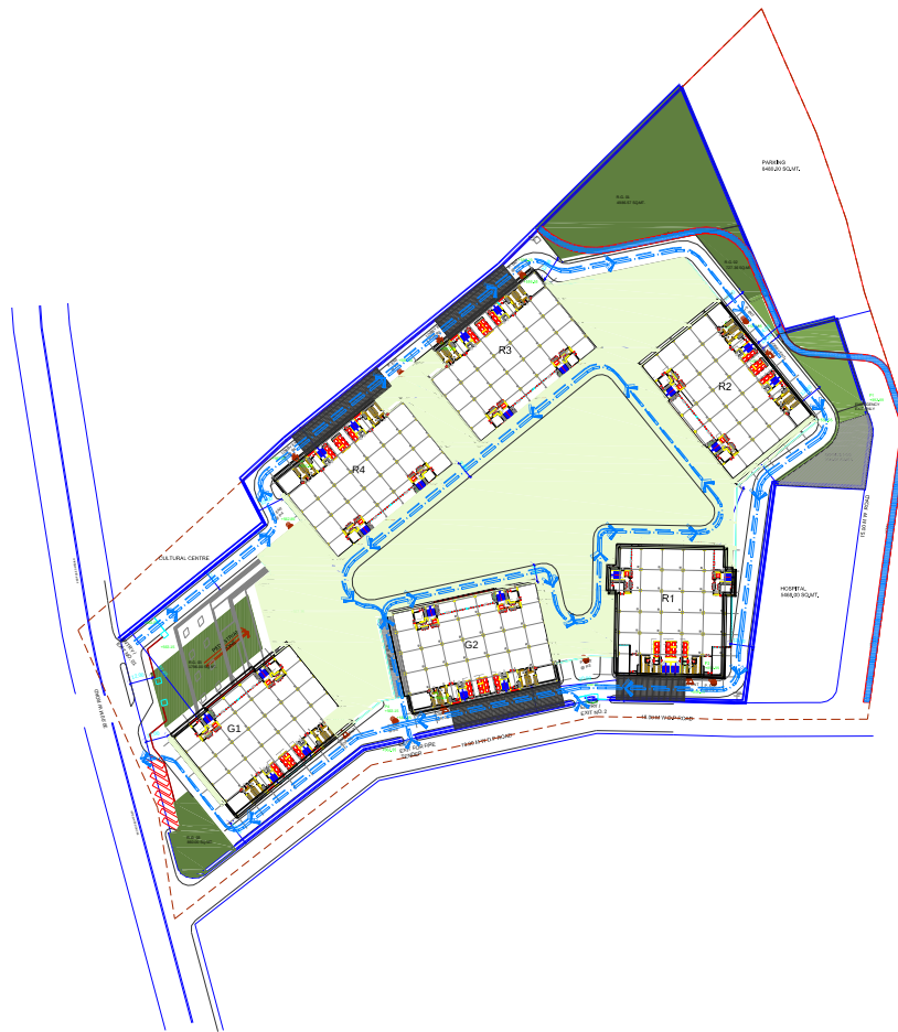
Figure 1.5 Fire tender Movement
